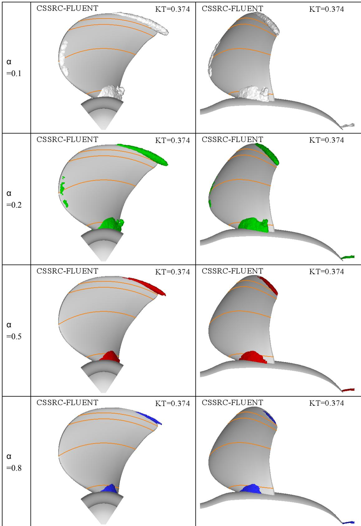
Figure 1 computed cavity shapes of case2-3-1( $\sigma=2.024$ )
