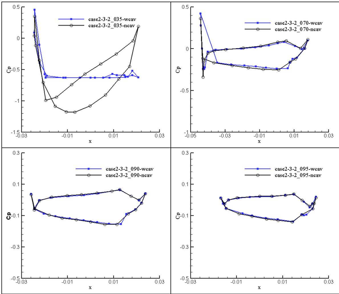
Figure 6 computed different radial section pressure coefficient of case2-3-2
