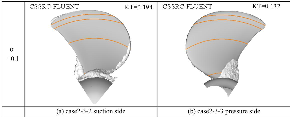
Figure 4 computed cavity shapes of case2-3-2 and case2-3-3
