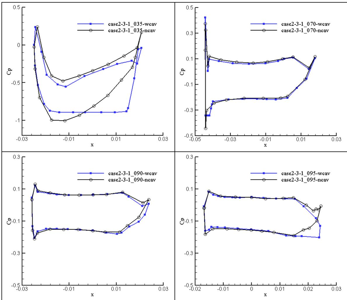
Figure 5 computed different radial section pressure coefficient of case2-3-1
