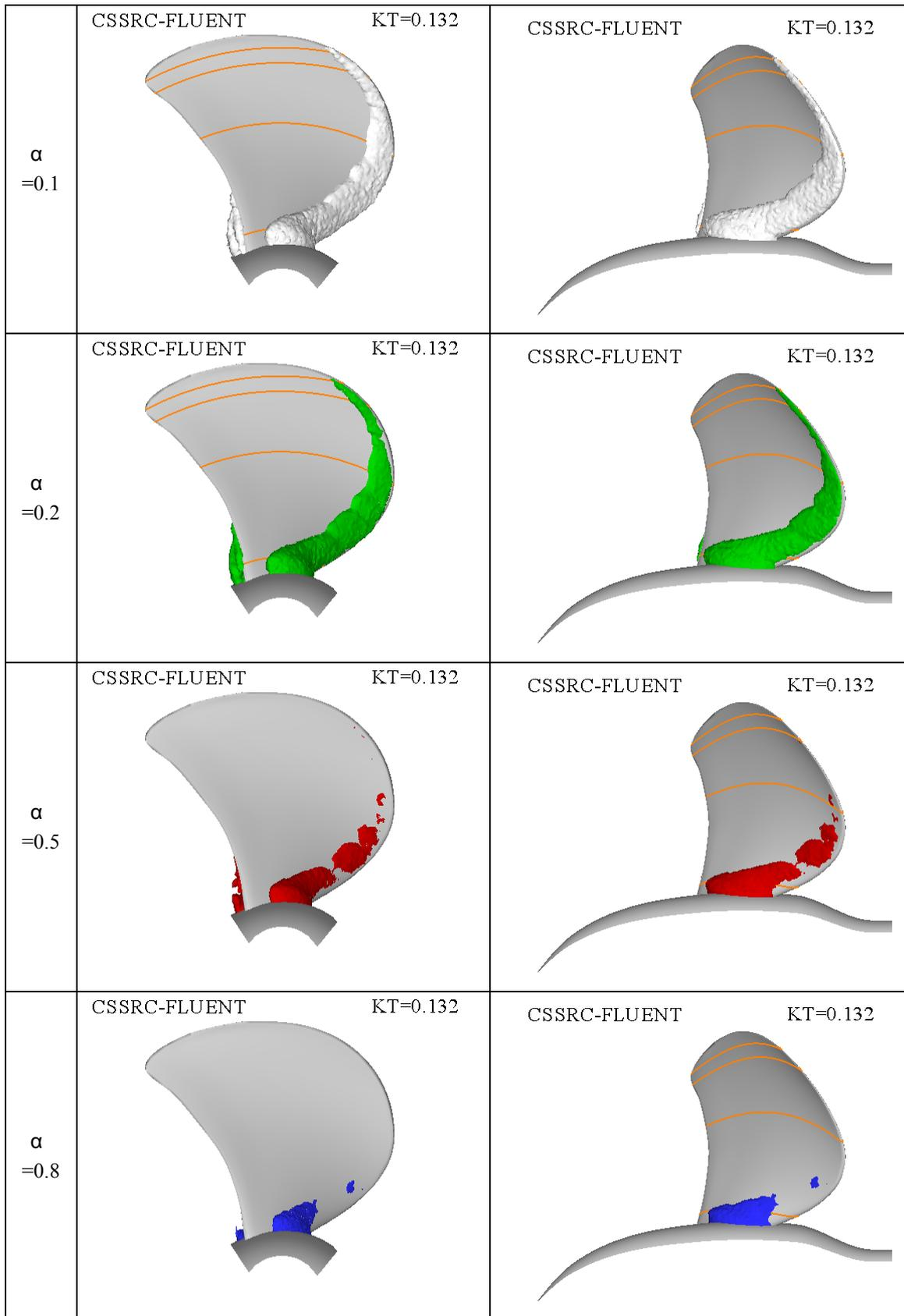
Figure 3 computed cavity shapes of case2-3-3( $\sigma=2.000$ )
