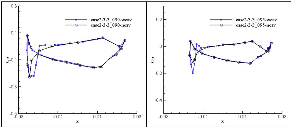
Figure 7 computed different radial section pressure coefficient of case2-3-3
