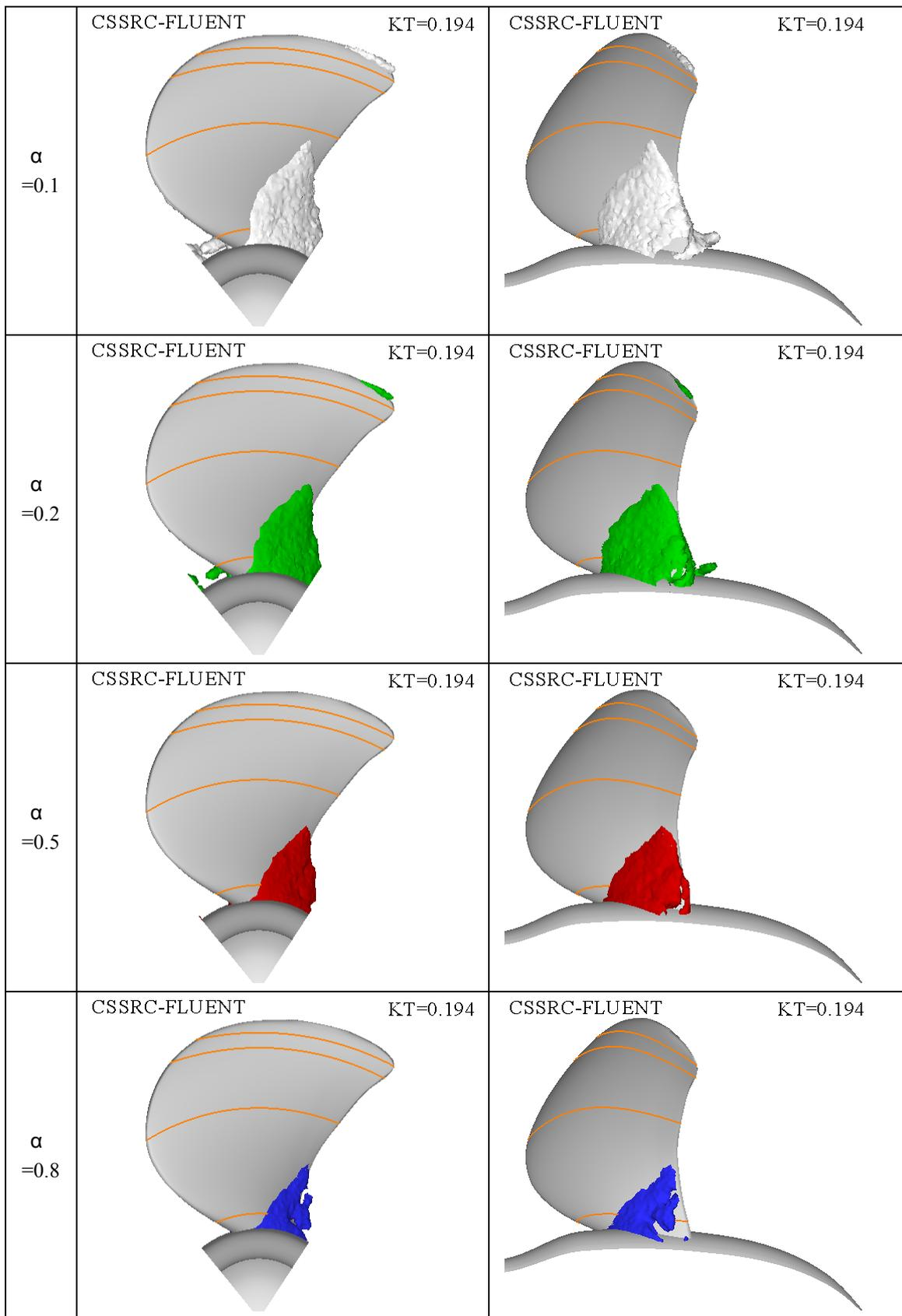
Figure 2 computed cavity shapes of case2-3-2( $\sigma=1.424$ )
