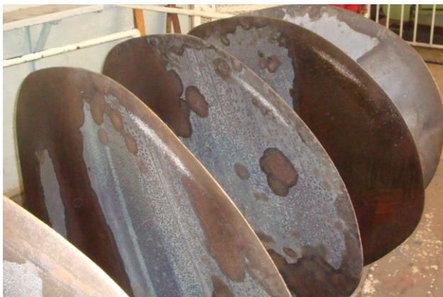
Figure 2: Cavitation damage on a dredger propeller
