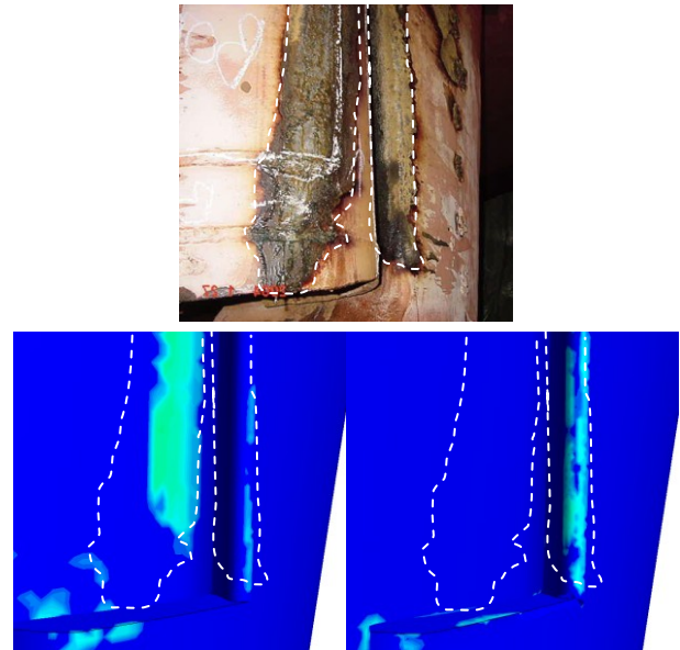
Figure 16: Cavitation erosion around gap between rudder and horn (top) and predicted erosive potential of flow as calculated when rudder is turned 4^\circ to starboard (left) and 4^\circ to port (right)
