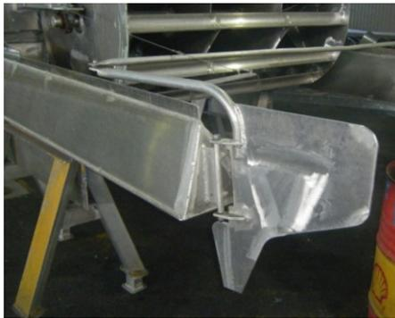
**Figure 2: Hull extensions and rudder modifications**
