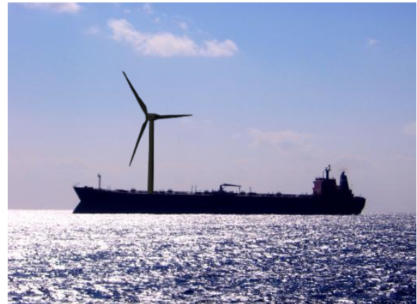
Figure 5: Illustration of a Vestas V39/600 wind turbine onboard a tanker for power generation.
