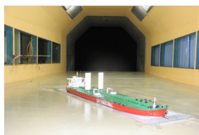
Figure 8 Wind tunnel model test for ship with two rear sails
