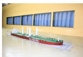
Figure 6 Wind tunnel model test for ship with four sails
