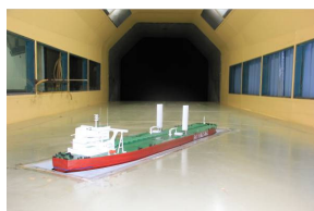
Figure 7 Wind tunnel model test for ship with two front sails
