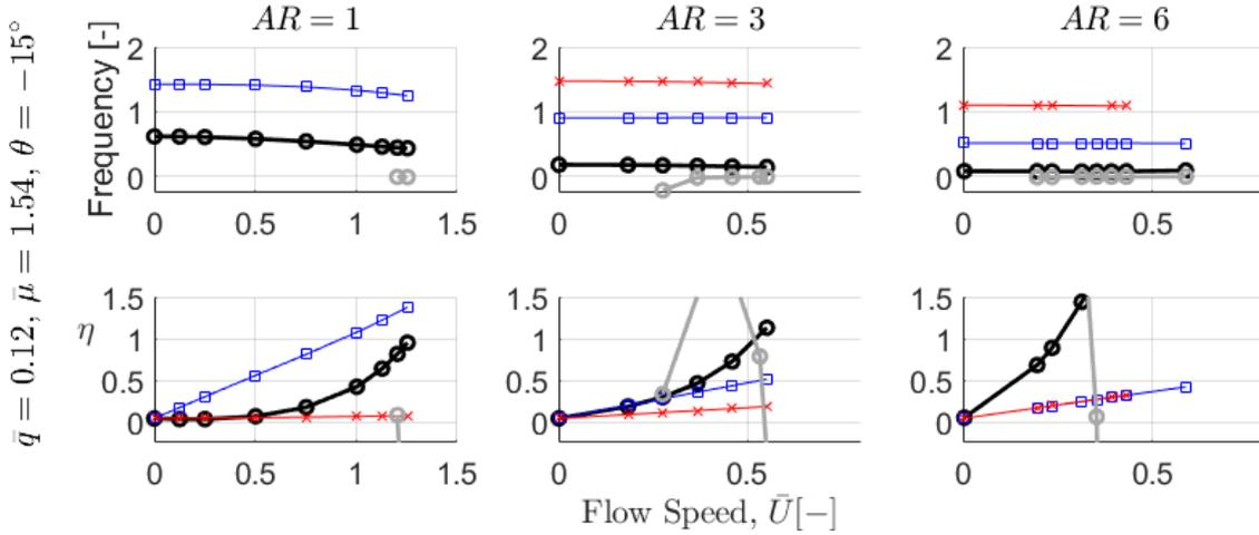
Figure 8: The effect of the aspect ratio  $AR$  and flow speed  $\bar{U}$  on the dimensionless natural frequencies and associated damping for fiber angle  $\theta = -15^\circ$  and in water.
