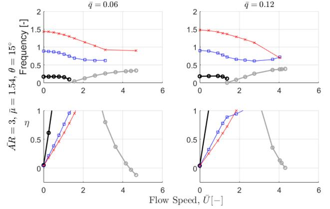
**Figure 5: The effect of nondimensional thickness ratio  $\bar{q}$  and flow speed  $\bar{U}$  on the dimensionless natural frequencies and associated damping for fiber angle  $\theta = 15^\circ$  and in water.**
