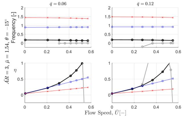
**Figure 6: The effect of nondimensional thickness ratio  $\bar{q}$  and flow speed  $\bar{U}$  on the dimensionless natural frequencies and associated damping for fiber angle  $\theta = -15^\circ$  and in water.**
