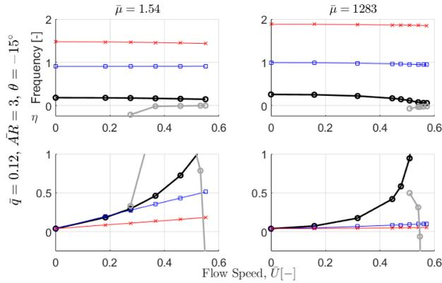
**Figure 4: The effect of nondimensional solid-to-fluid density ratio  $\bar{\mu}$  and flow speed  $\bar{U}$  on the dimensionless natural frequencies and associated damping for fiber angle  $\theta = -15^\circ$ .**
