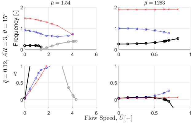
**Figure 3: The effect of nondimensional solid-to-fluid density ratio  $\bar{\mu}$  and flow speed  $\bar{U}$  on the dimensionless natural frequencies and associated damping for fiber angle  $\theta = 15^\circ$ .**
