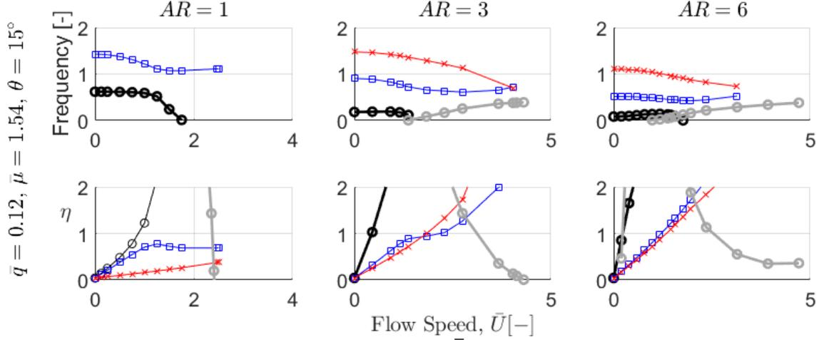
Figure 7: The effect of the aspect ratio  $AR$  and flow speed  $\bar{U}$  on the dimensionless natural frequencies and associated damping for fiber angle  $\theta = 15^\circ$  and in water.
