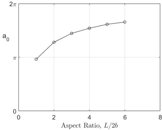
**Figure 2: The effect of the aspect ratio  $L/2b$  on the slope of the 3-D lift coefficient  $a_0$  at steady-state hydroelastic analysis of a rigid hydrofoil.**
