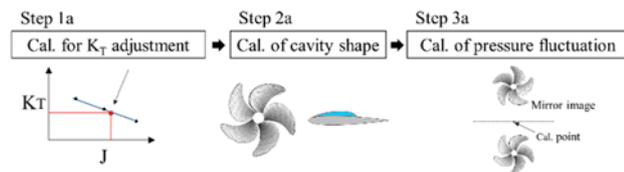
**Figure 1:** Series of calculation (Previous method)
