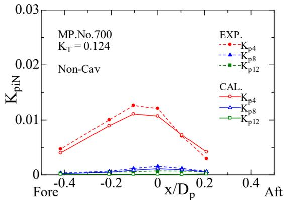
**Figure 10:** Amplitude distribution of pressure fluctuation of M.P.No.700 (Non-Cav, Longitudinal direction)
