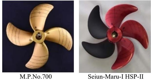
**Figure 3:** Model propellers
