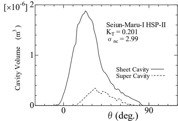
Figure 18: Calculated cavity volume of Seiun-Maru-I HSP-II
