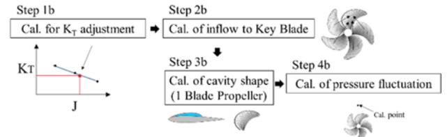
**Figure 2:** Series of calculation (Present method)
