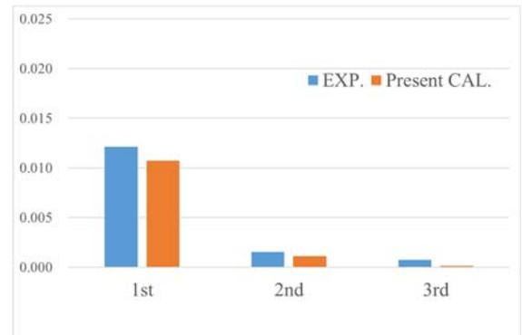
**Figure 14:** Amplitude of pressure fluctuation  $K_{piN}$  at P3 (M.P.No.700, Non-Cav,  $K_T=0.124$ ,  $\sigma_{nc}=1.37$ )
