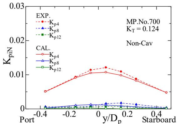
**Figure 11:** Amplitude distribution of pressure fluctuation of M.P.No.700 (Non-Cav, Transverse direction)
