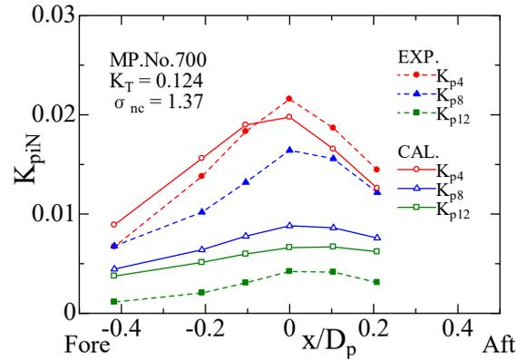
**Figure 12:** Amplitude distribution of pressure fluctuation of M.P.No.700 (w/Cav, Longitudinal direction)
