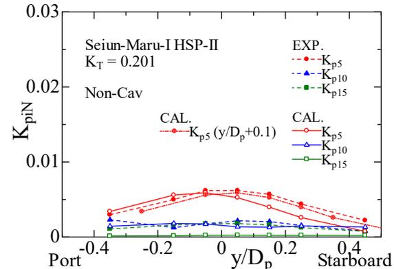
Figure 19: Amplitude distribution of pressure fluctuation of Seiun-Maru-I HSP-II (Non-Cav, Transverse direction)
