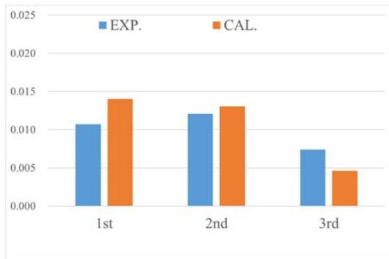
**Figure 22:** Amplitude of pressure fluctuation  $K_{piN}$  at P3 (Seiu-Maru-I HSP-II, w/Cav,  $K_T=0.201$ ,  $\sigma_{nc}=2.99$ )
