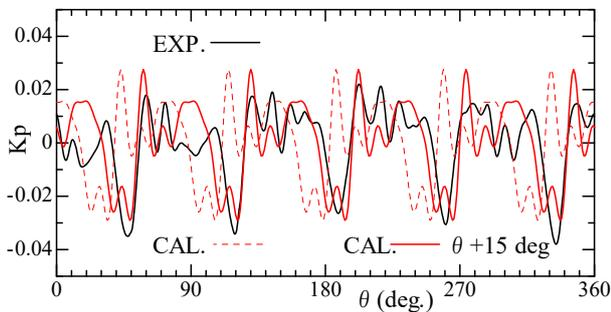
**Figure 23:** Fluctuating pressure in one revolution at P3 (Seiu-Maru-I HSP-II, w/Cav,  $K_T=0.201$ ,  $\sigma_{nc}=2.99$ )
