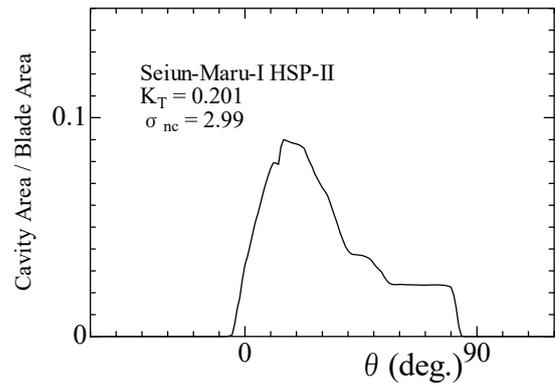
Figure 17: Calculated cavity area of Seiun-Maru-I HSP-II
