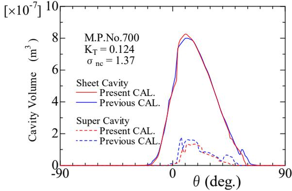
**Figure 9:** Calculated cavity volume of M.P.No.700
