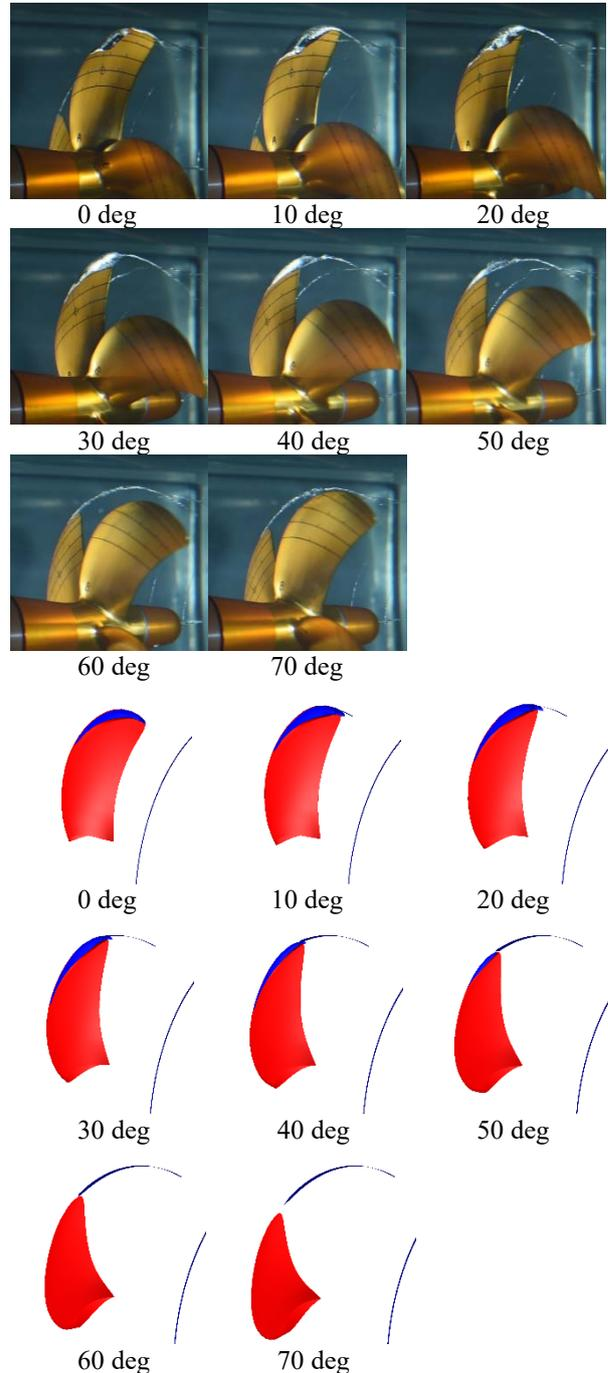
**Figure 7:** Cavitation patterns of M.P.No.700 ( $K_T=0.124$ ,  $\sigma_{nc}=1.37$ , upper:EXP., lower:CAL.)
