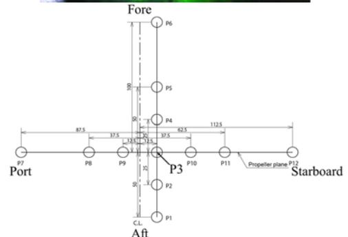
**Figure 5:** Location of pressure transducer on flat plate
