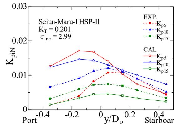
Figure 20: Amplitude distribution of pressure fluctuation of Seiun-Maru-I HSP-II (w/Cav, Transverse direction)
