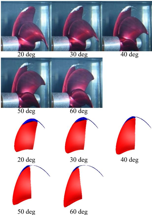
Figure 16: Cavitation patterns of Seiun-Maru-I HSP-II ( $K_T=0.201$ ,  $\sigma_{nc}=2.99$ , upper:EXP., lower:CAL.)
