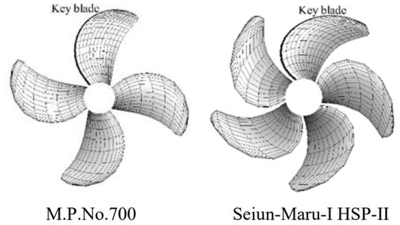
**Figure 4:** Panel arrangements for cavitation model
