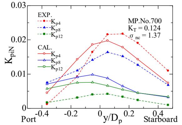
**Figure 13:** Amplitude distribution of pressure fluctuation of M.P.No.700 (w/Cav, Transverse direction)
