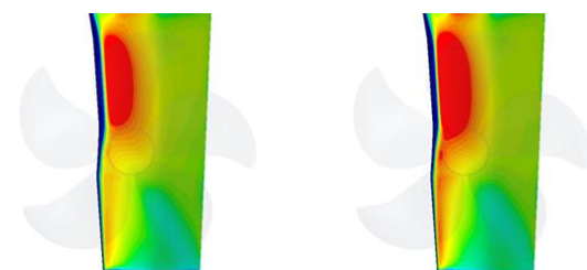
Figure 24 Instantaneous pressure distributions on rudder during STBD turning (looking downstream)
