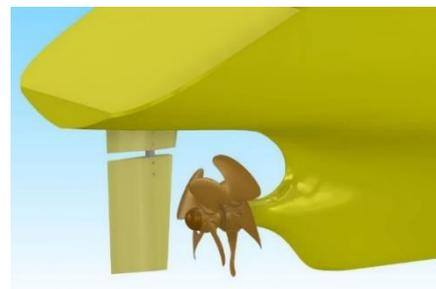
Figure 1. Contra Rotating Propeller.
