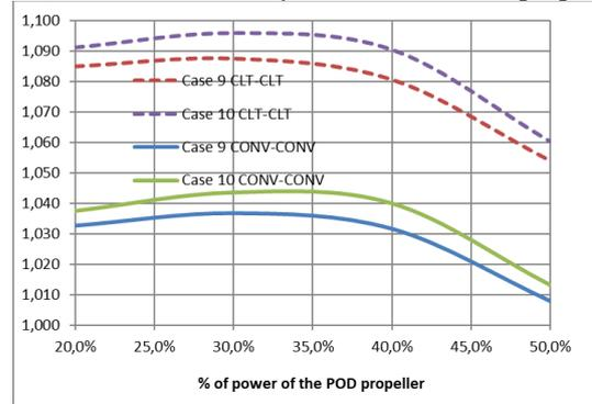
**Figure 13. Energy saving in LNG ships.**
