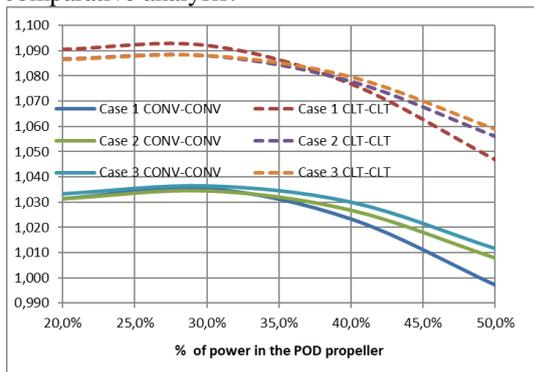
**Figure 11. Energy saving in Oil tankers.**
