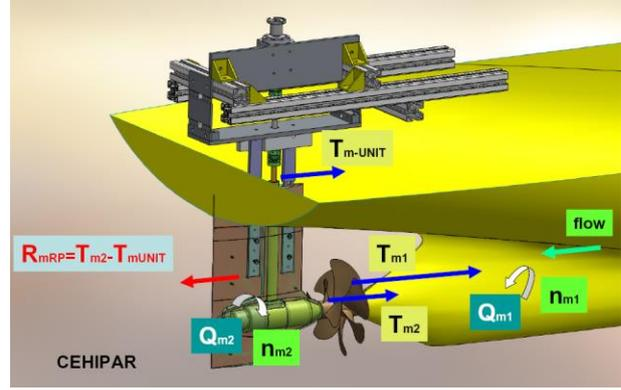
Figure 6. Self-propulsion test scheme.
