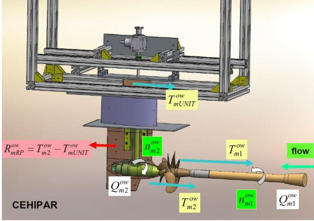
Figure 5. Open water test device.
