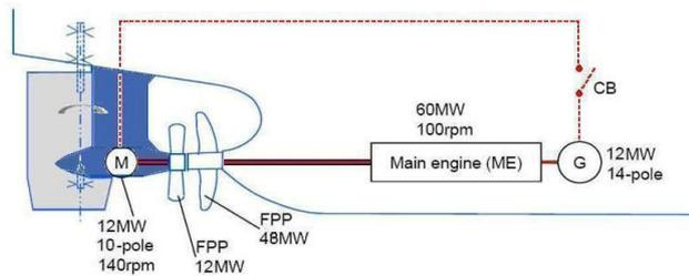
**Figure 4. CRP-POD configuration.**
