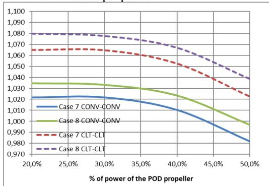
**Figure 12. Energy saving in Container ships.**
