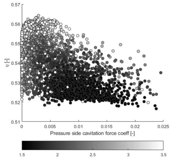
Figure 3 Pressure side cavitation force coefficient and efficiency, colored by 1<sup>st</sup> order pressure pulse
