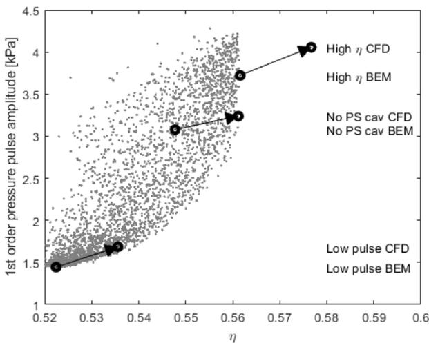
Figure 8 Pareto front from the BEM-based optimization and the predicted performance for three individuals using CFD
