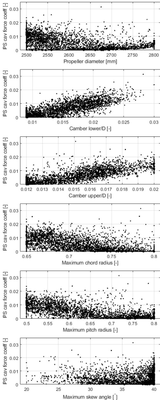
Figure 6 Parameter influence on pressure side cavitation force coefficient
