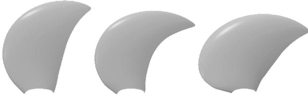
Figure 4 Selected individuals for high fidelity CFD analysis. High efficiency design (left), no pressure side cavitation design (center) and low pressure pulse design (right)
