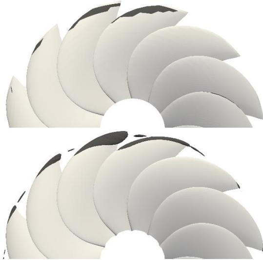
Figure 9 Blade pressure and cavitation every 30°, BEM (top) and CFD (bottom) for high efficiency design
