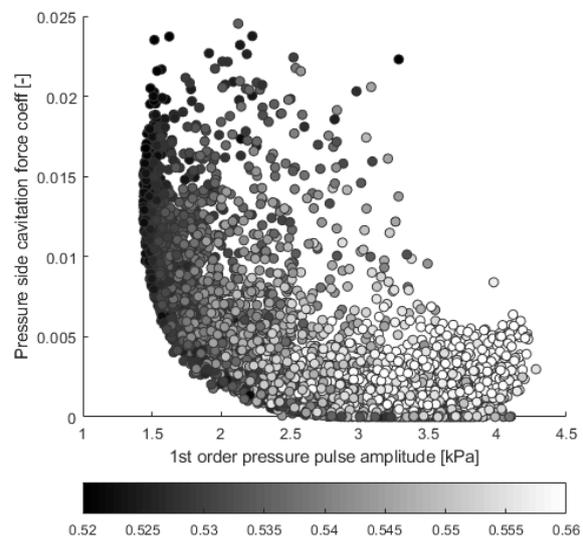
Figure 2 1<sup>st</sup> order pressure pulse and pressure side cavitation force coefficient, colored by efficiency
