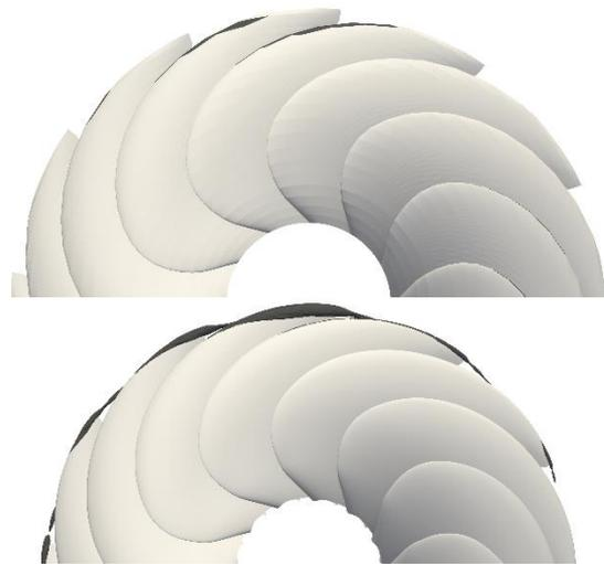
Figure 11 Blade pressure and cavitation every 30°, BEM (top) and CFD (bottom) for low pulse design
