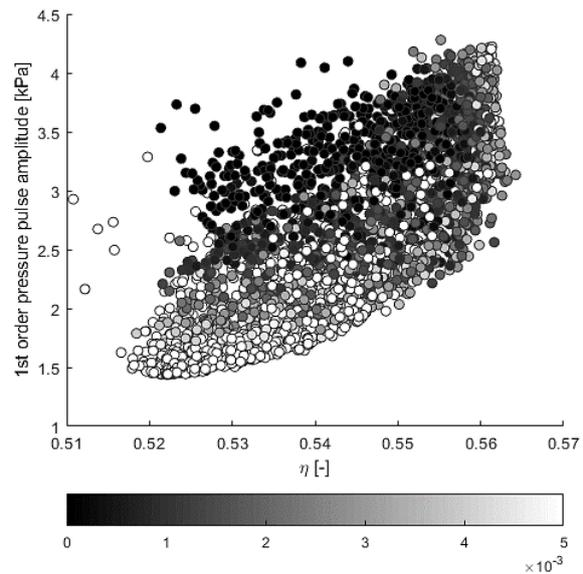
Figure 1 Efficiency and 1<sup>st</sup> order pressure pulse, colored by pressure side cavitation force coefficient
