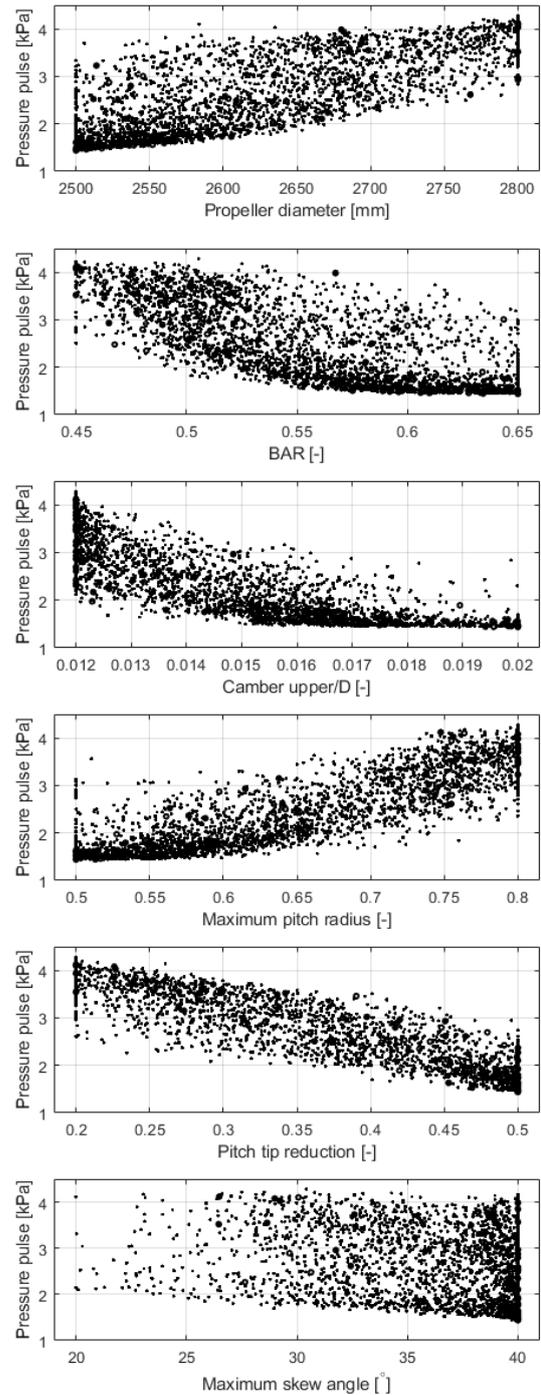
Figure 7 Parameter influence on 1st order pressure pulse amplitude
