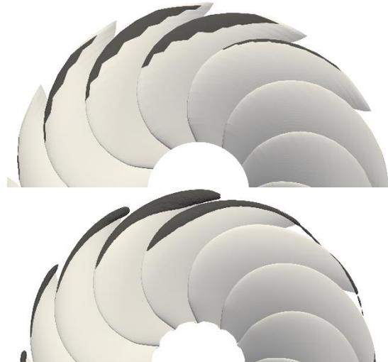
Figure 10 Blade pressure and cavitation every 30°, BEM (top) and CFD (bottom) for no pressure side cavitation design
