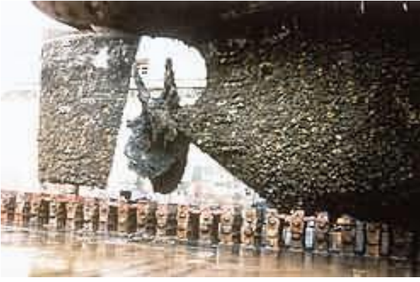
Figure 2 Vessel with Severe Fouling
