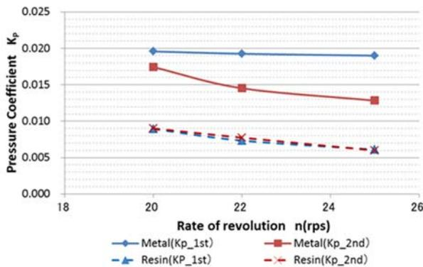
Figure 6 Comparison of pressure fluctuations ( $K_T=0.201$ ).
