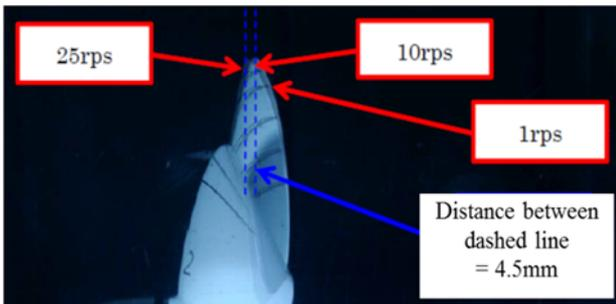
Figure 3 Behavior of resin propeller deformation ( $J=0.6$ ).
