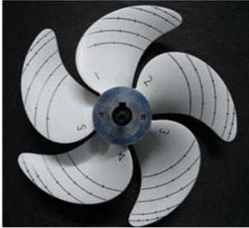
**Figure 1 Flexible composite highly skewed model propeller HSP-II of "SEIUN-MARU I".**
