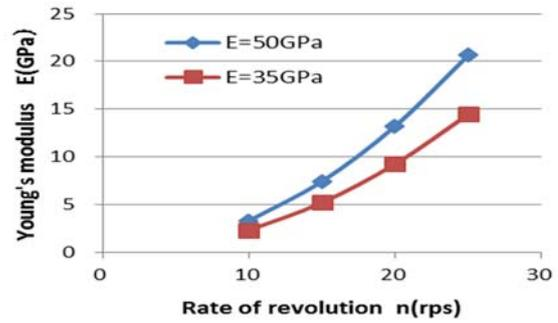
Figure 12 Necessary Young's modulus for model propeller.
