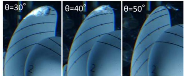
Figure 9 Comparison of cavitation patterns for resin propeller ( $K_T=0.201$ ,  $n=25\text{rps}$ ).
