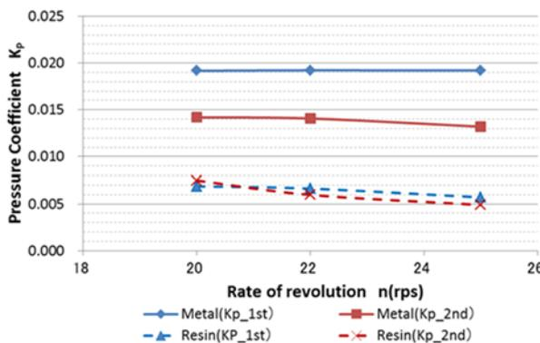
Figure 7 Comparison of pressure fluctuations ( $\sqrt{K_T/J}=0.626$ ).
