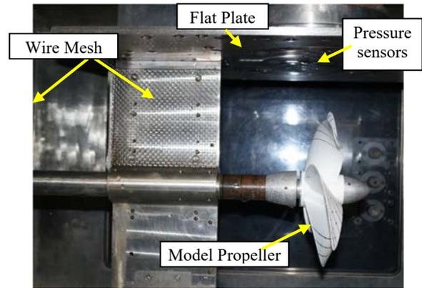
**Figure 2 Test arrangements in cavitation tunnel.**
