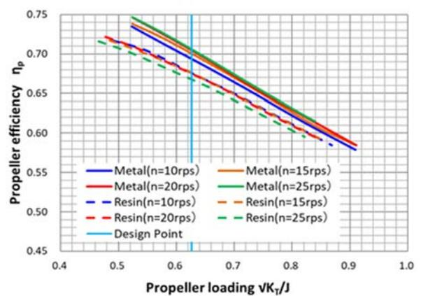
Figure 4 Comparison of propeller open water characteristics in uniform flow.
