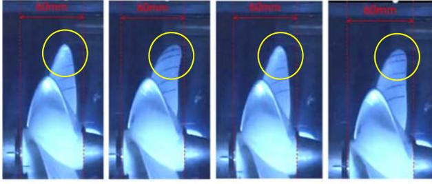
Figure 11 Unsteady deformation of the foil at the time of propeller reverse in wake ( $J = -0.4$ ,  $n = -10$ rps).
