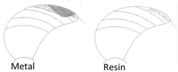
Figure 8 Comparison of cavitation patterns ( $K_T=0.201$ ,  $n=25\text{rps}$ ,  $\theta=40^\circ$ ).
