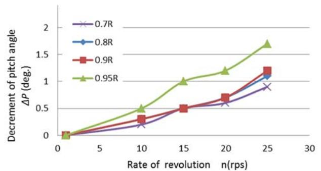
Figure 10 Comparison of decrement of pitch angle for resin propeller ( $K_T=0.201$ ,  $\theta=300^\circ$ ).
