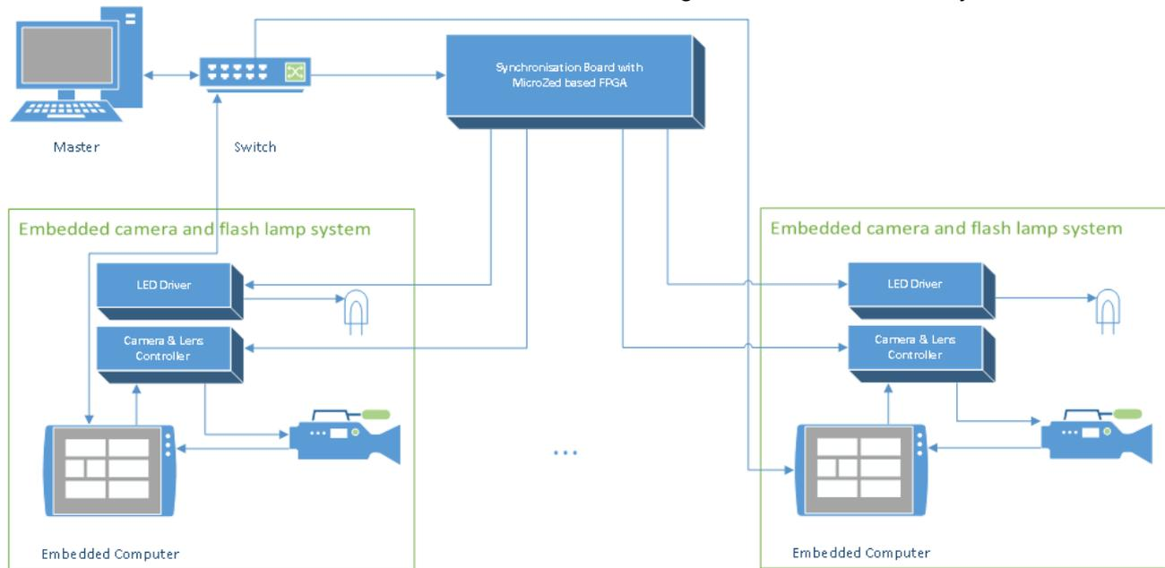
Figure 1: Subcomponents of the recording system
