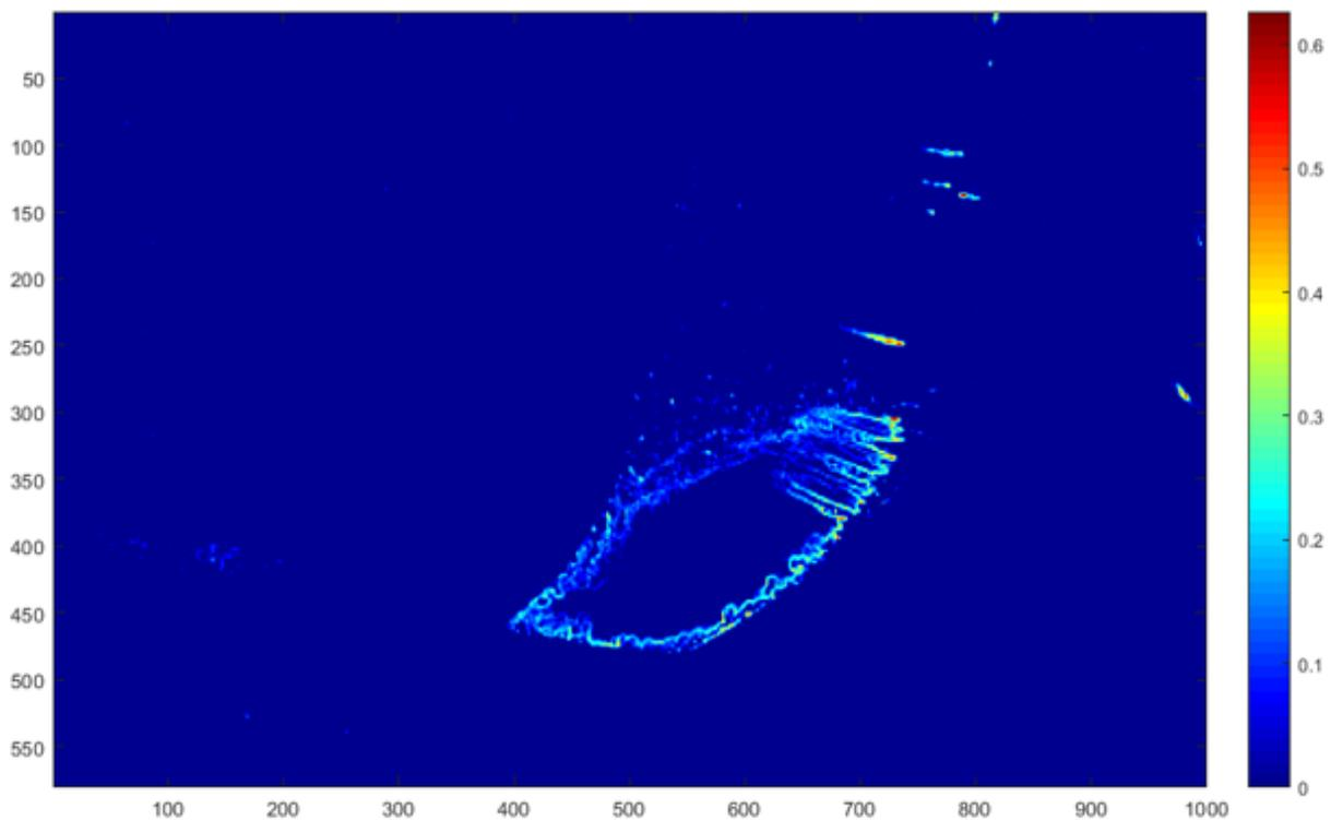
Figure 6: Histogram like occurrence statistics of sheet cavitation based on closed point chains of 22 images
