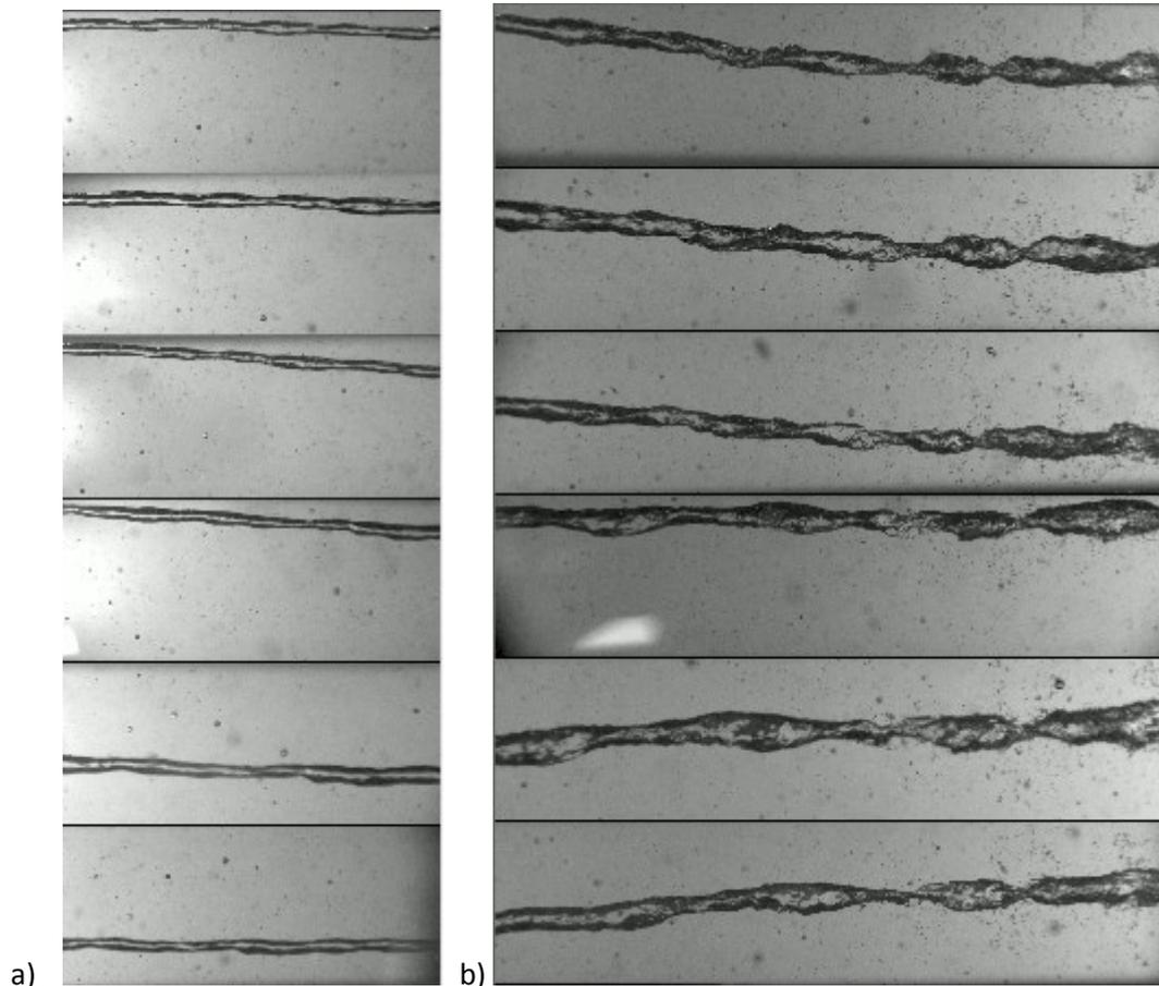
Figure 3: Tip-Vortex from 12 different viewpoints recorded at the University of Rostock K21 cavitation tunnel at 5 m/s, 9 deg angle of the foil and 500 mbar pressure a) depicts results from first ring and b) depicts the second ring synchronized images.
