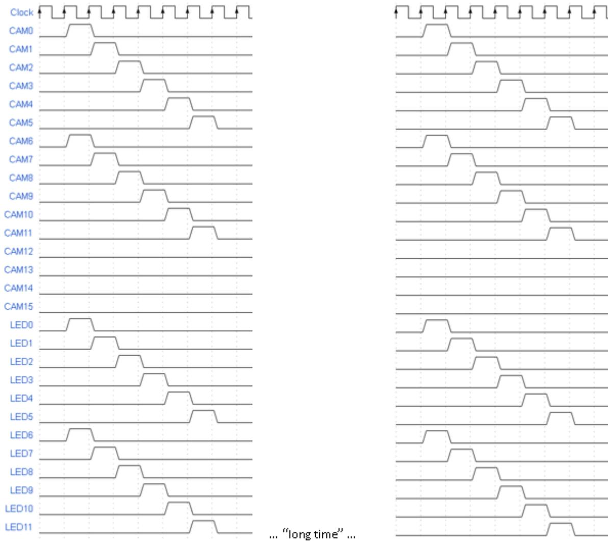
Figure 4: Timing Diagram (clock cycle is  $37\mu\text{s}$ ) of the applied FPGA trigger system based on AVnet Micro-Zed 7020 (“long time” means in case of the depicted recording approx. 20ms for 50 frames per second)
