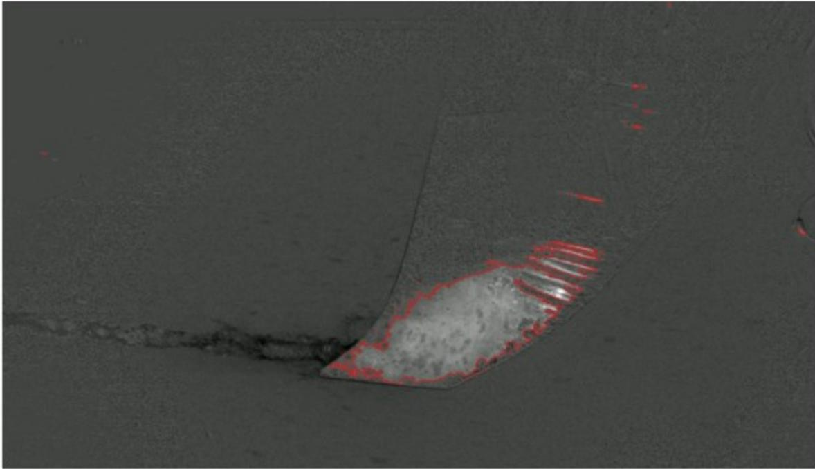
Figure 5: Example of automatic segmented sheet cavitation form a sample in University of Rostock K21 cavitation canal at 5 m/s, 9 deg angle of the hydrofoil and 500 mbar pressure.
