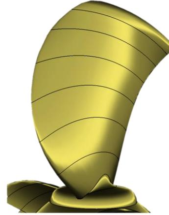
Figure 3. Division of propeller blade in strips.
