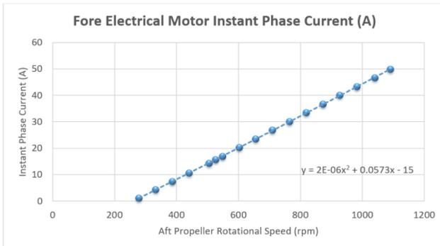
**Figure 8 Fore Electrical Motor Instant Phase Current vs Aft Propeller Rotational Speed**
