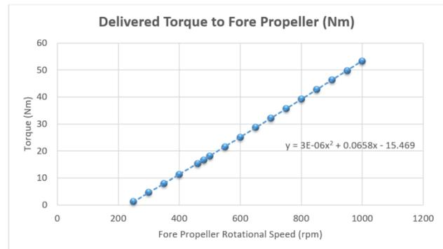
**Figure 5 Delivered Torque to Fore Propeller vs Fore Propeller Rotational Speed**
