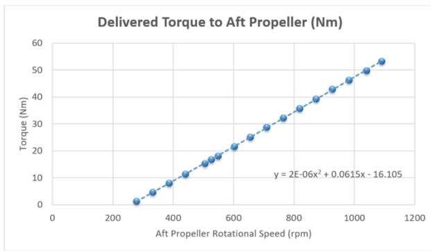
**Figure 7 Delivered Torque to Aft Propeller vs Aft Propeller Rotational Speed**
