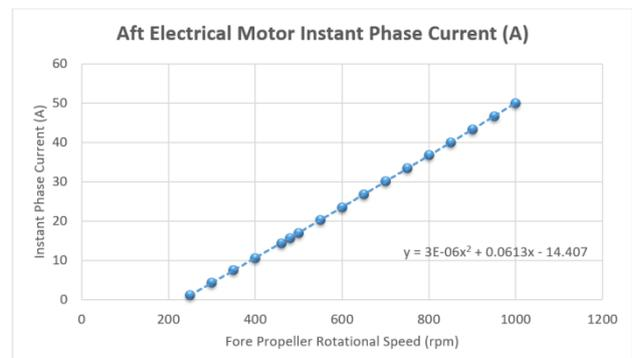
**Figure 6 Aft Electrical Motor Instant Phase Current vs Fore Propeller Rotational Speed**
