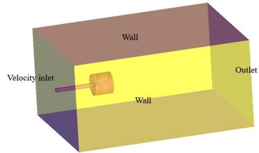
**Figure 2 Calculation domain of single propeller**
