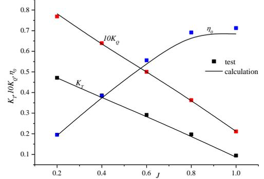
Figure 5 Open water hydrodynamic performance of propeller
