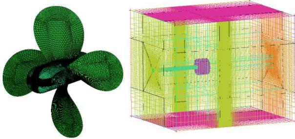
(a) Grids of propeller (b) Grids of external domain
