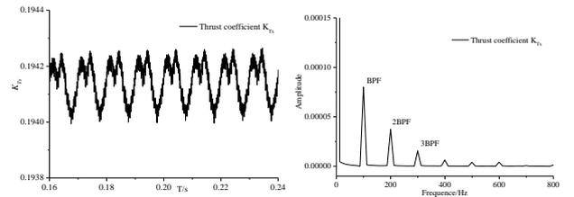
(a) Time-domain data of  $K_{Tx}$  (b) Frequency-domain data of  $K_{Tx}$
