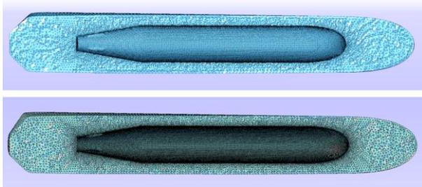
**Figure 6. Axial force in simulation calculated on body by different mesh types and representation of coarse & medium mesh**
