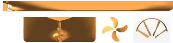
**Figure 1 The bulk tanker and propeller model**
