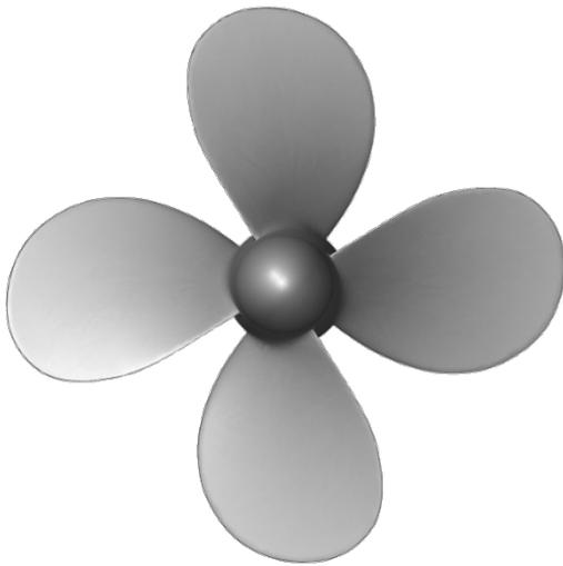
Figure 1: INSEAN E779A propeller geometry
