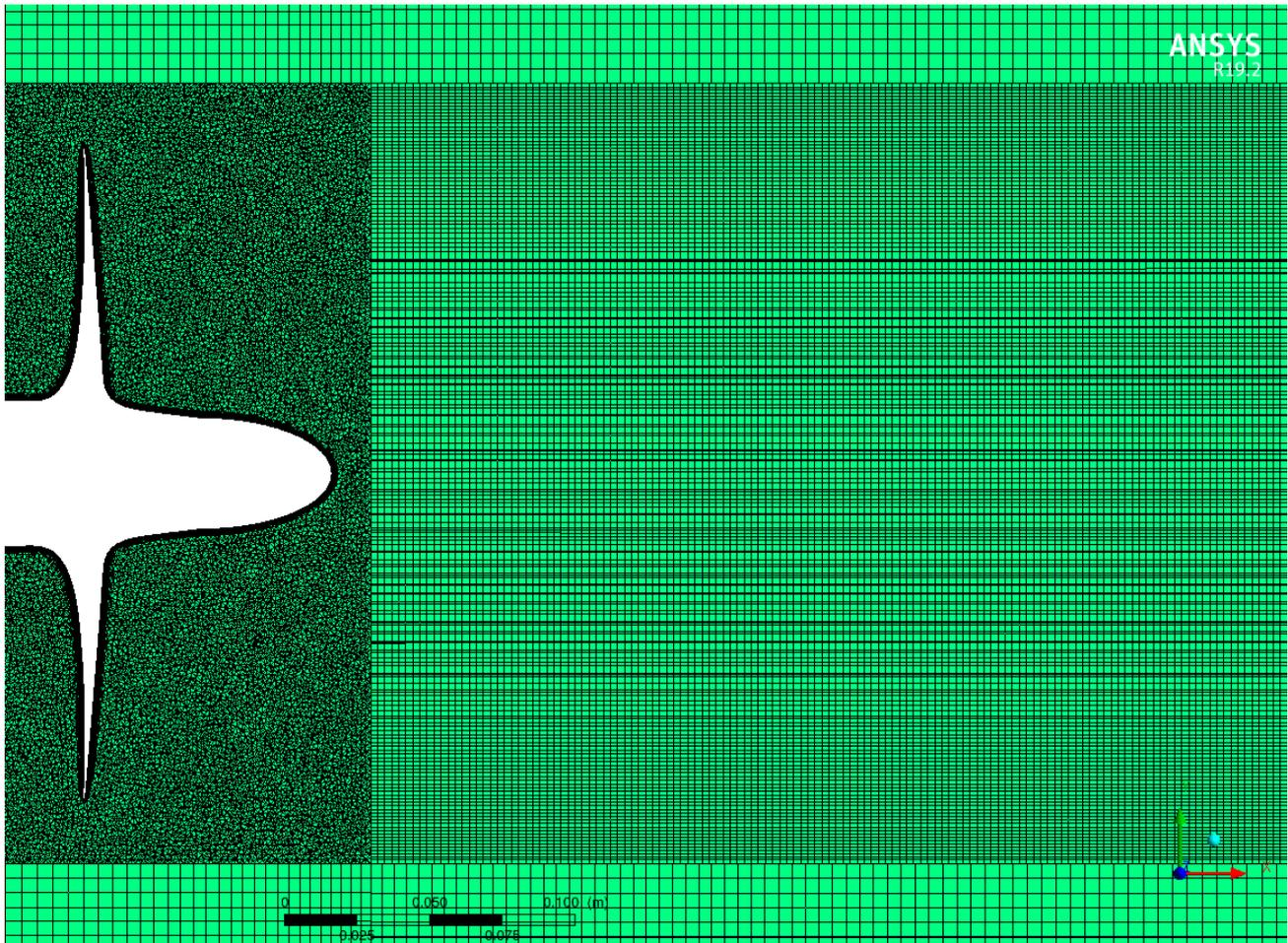
Figure 3: Mesh on the mid-longitudinal plane  $XY$
