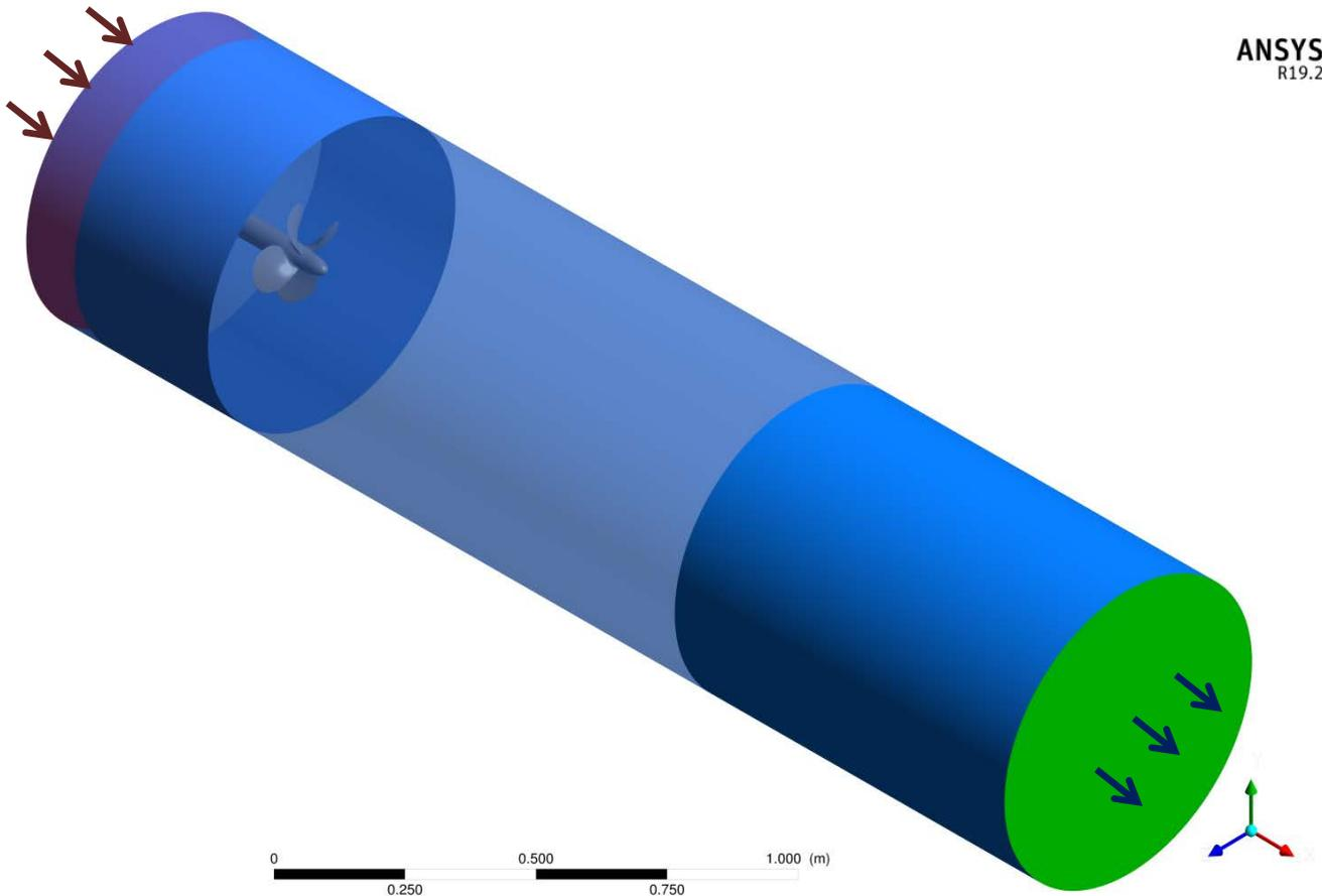
Figure 2: Computational domain and boundary Conditions
