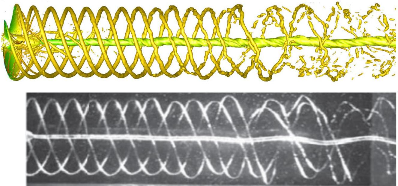
**Figure 4: Comparison of wake vortical structures between LES and experiments (Felli et al 2011)**
