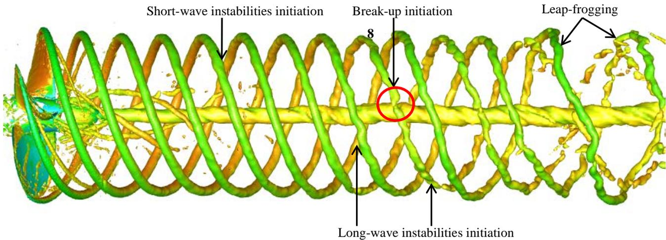
Figure 6: Instabilities in the wake vortical structures (colored by axial velocity)
