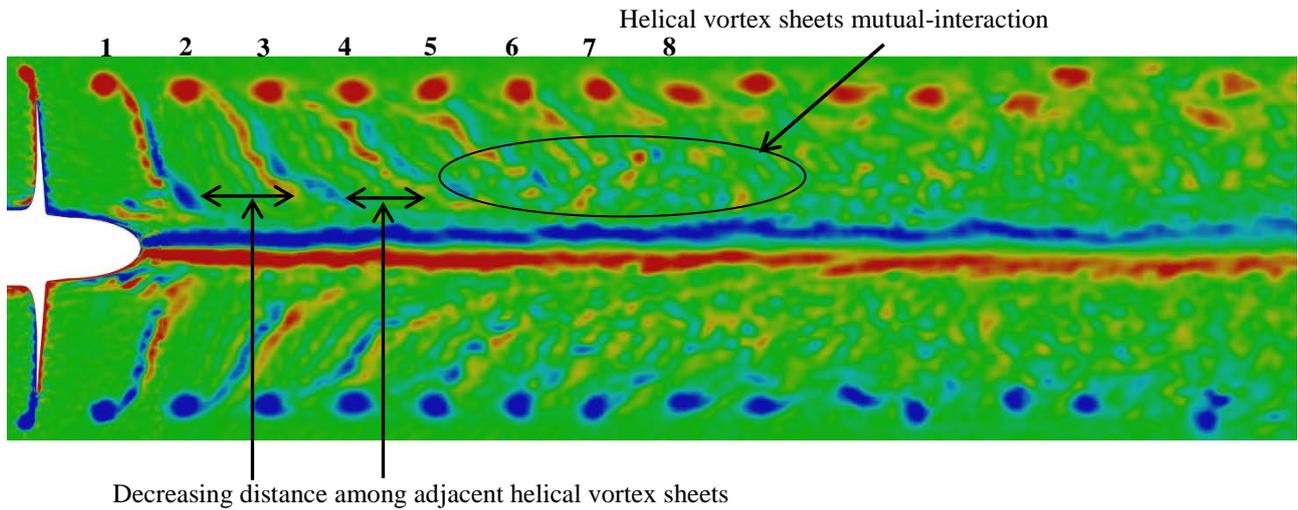
Figure 5: Out-of-plane vorticity contours on the mid-longitudinal plane
