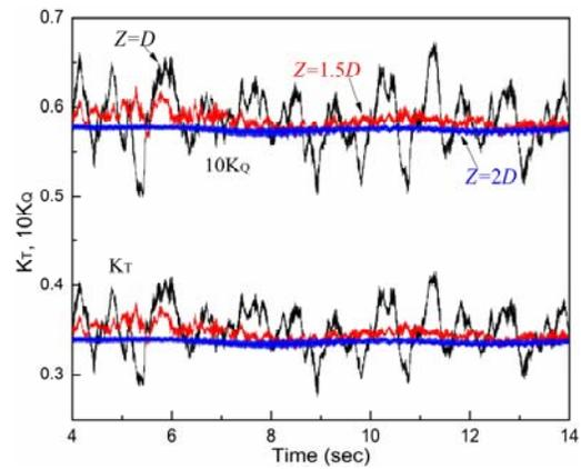
Figure 15: Time histories of thrust and torque coefficients.
