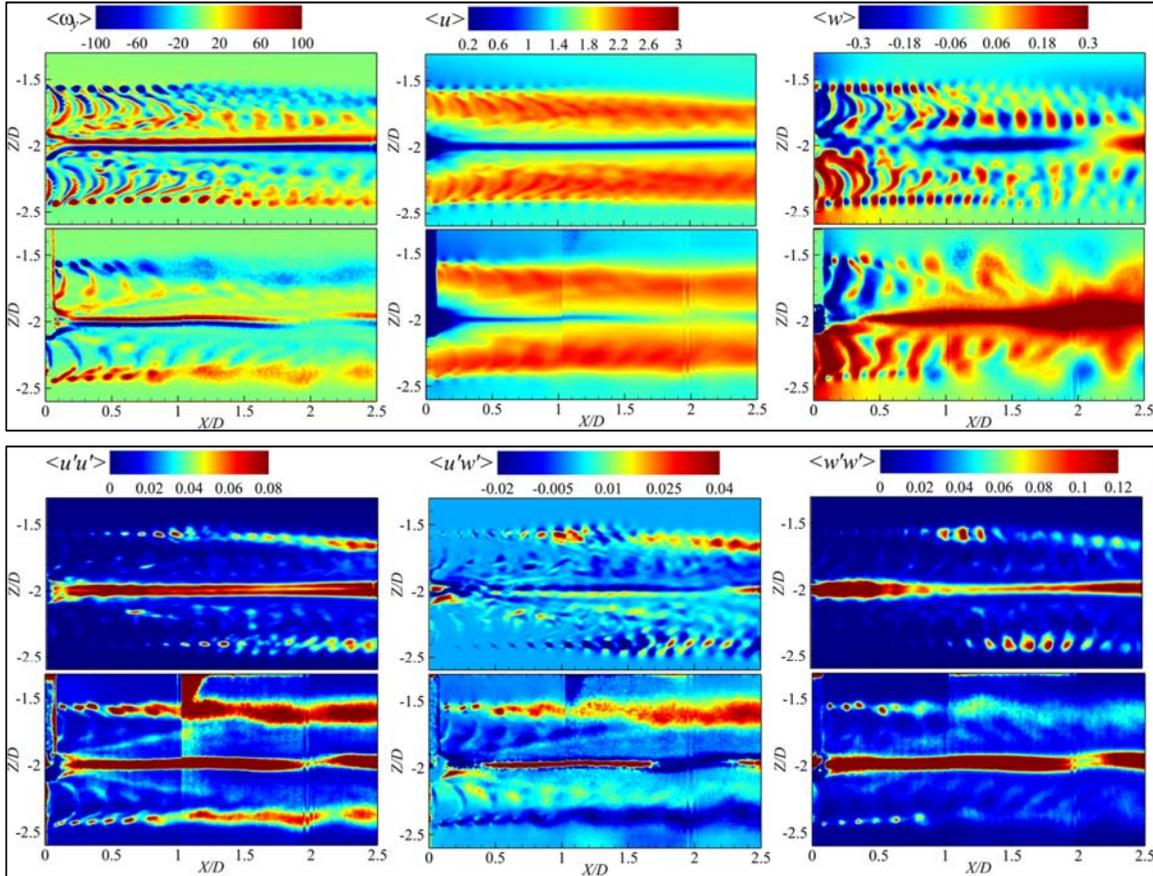
Figure 7: Phase averaged flow quantities for  $J = 0.82$ ,  $U = 1.5$  m/s,  $Z = 2D$ . Each panel top: CFD, bottom: EFD.
