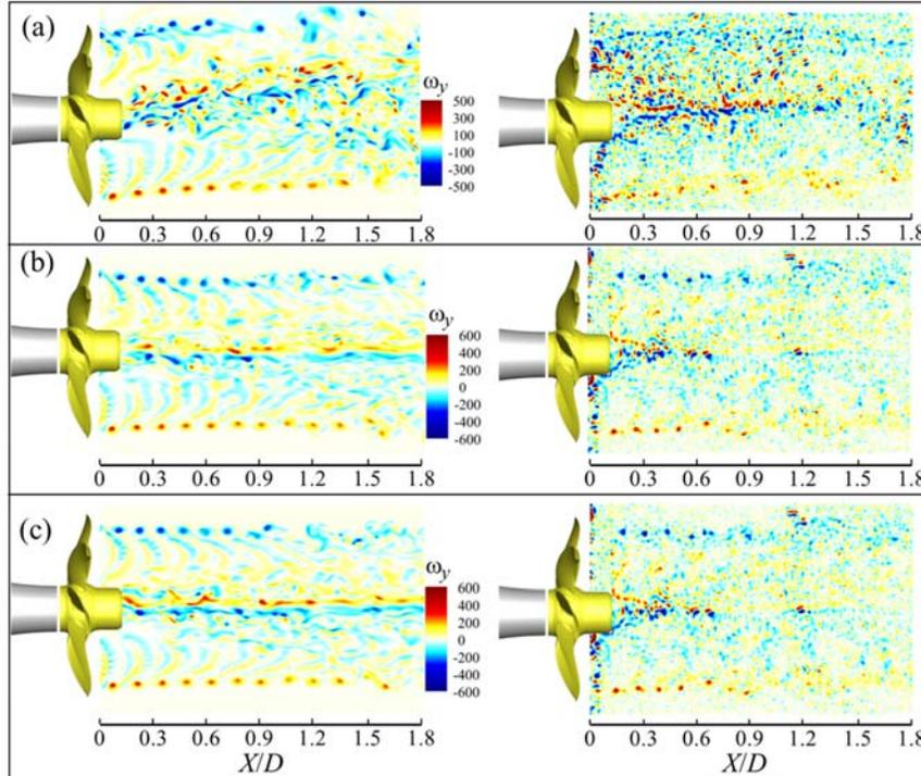
Figure 8: Snapshots of vorticity for  $Z/D = 1$  (a),  $Z/D = 1.5$  (b), and  $Z/D = 2$  (c). Left: CFD, right: EFD.
