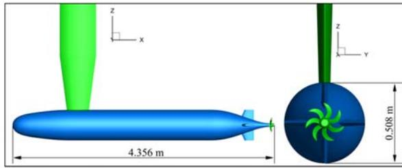
Figure 1: DARPA Suboff fitted with E1658 propeller.
