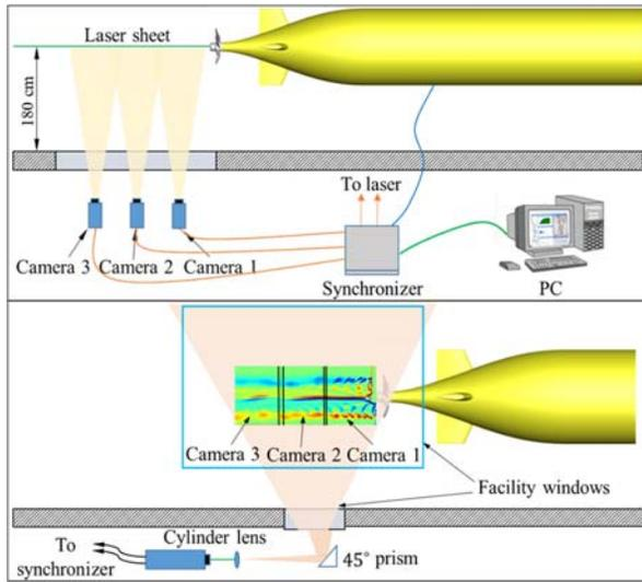
Figure 2: Top and side views of the experimental set-up.
