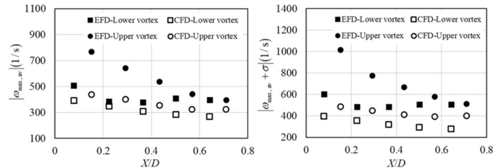
Figure 12: Tip vortex strength (computed as  $\omega_{\max, av}$  and  $\omega_{\max, av} + \sigma$ ) for  $J = 0.82$ ,  $U = 1.5$  m/s,  $Z = 1.5D$ .
