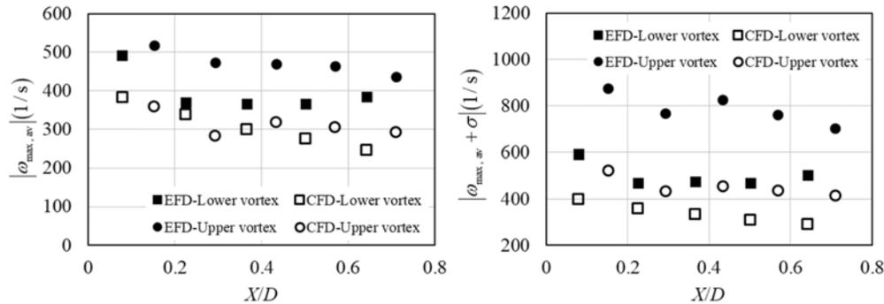
Figure 11: Tip vortex strength (computed as  $\omega_{\max, av}$  and  $\omega_{\max, av} + \sigma$ ) for  $J = 0.82$ ,  $U = 1.5$  m/s,  $Z = D$ .
