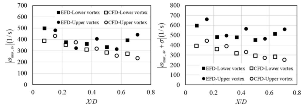
Figure 13: Tip vortex strength (computed as  $\omega_{\max, av}$  and  $\omega_{\max, av} + \sigma$ ) for  $J = 0.82$ ,  $U = 1.5$  m/s,  $Z = 2D$ .
