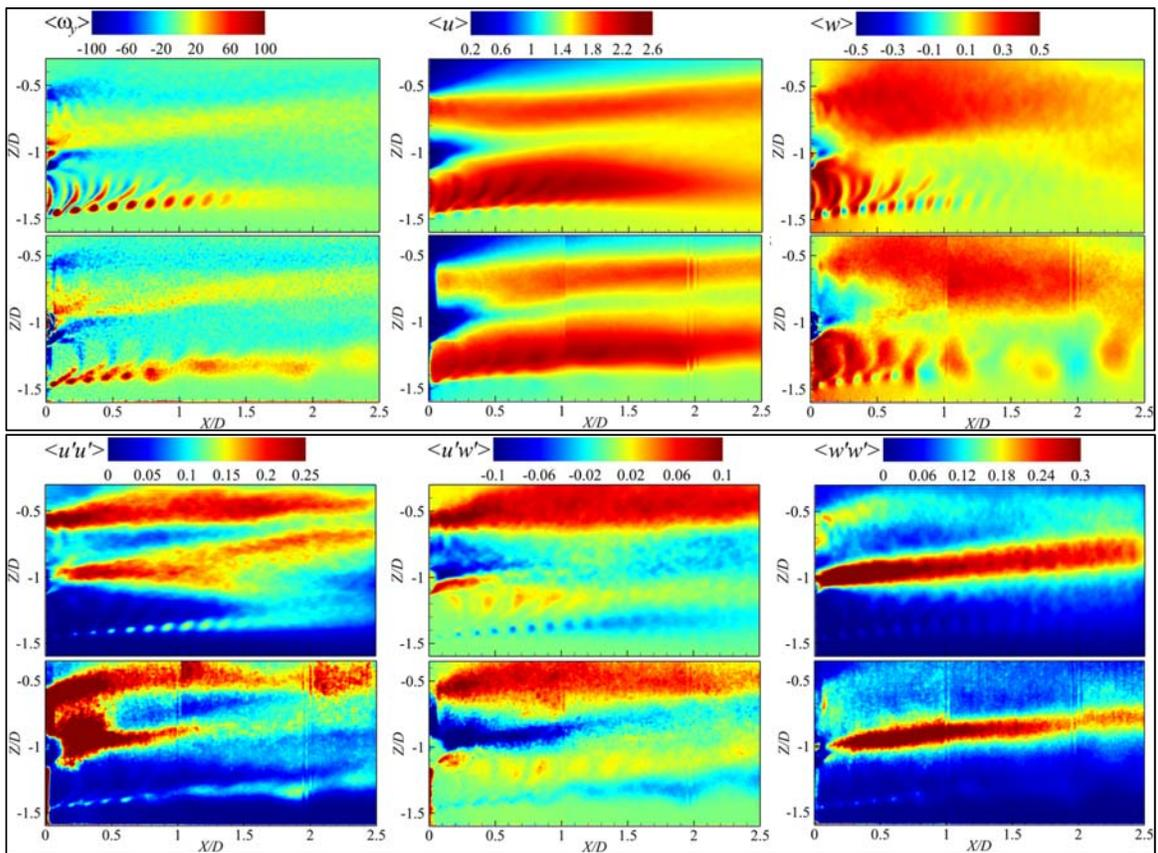
Figure 5: Phase averaged flow quantities for  $J = 0.82$ ,  $U = 1.5$  m/s,  $Z = D$ . Each panel top: CFD, bottom: EFD.
