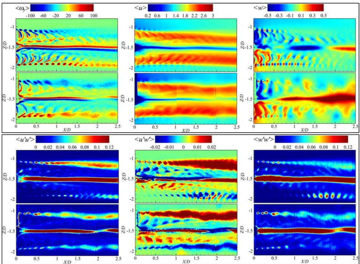
Figure 6: Phase averaged flow quantities for  $J = 0.82$ ,  $U = 1.5$  m/s,  $Z = 1.5D$ . Each panel top: CFD, bottom: EFD.
