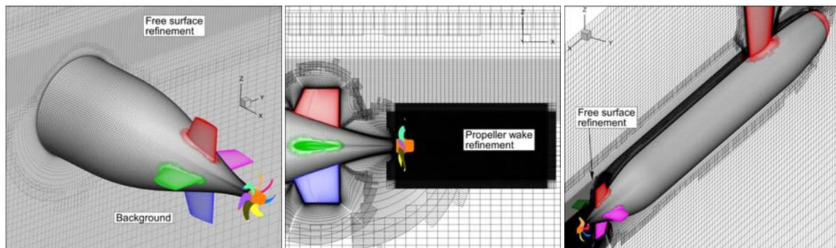
Figure 3: Overset grid system with free surface refinement and propeller wake refinement
