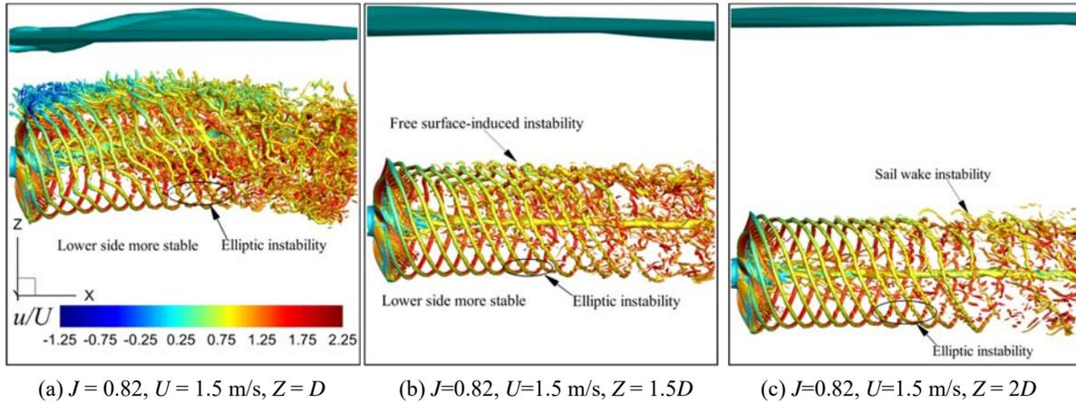
Figure 4: Instantaneous views of the wake of the propeller represented by isosurfaces of  $Q = 30000$  for three shaft depths.
