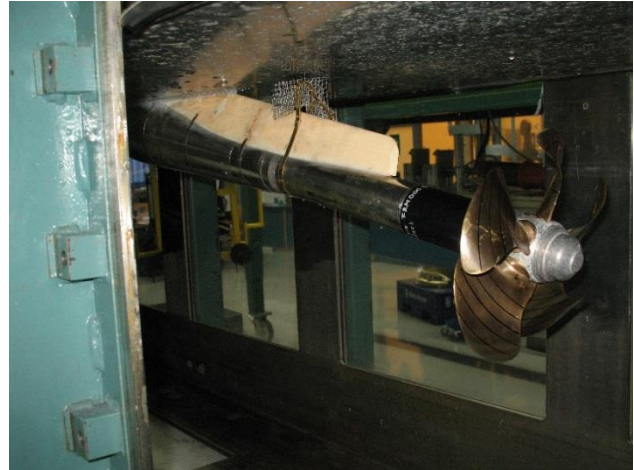
Figure 6: Propeller, shaft and wake generating mesh inside the cavitation tunnel.
