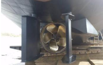
Figure 4: Final propeller mounted on the ship, the duct is part of the hull.
