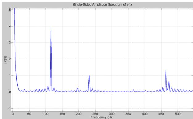
Figure 10. Single-sided Amplitude Spectrum of Fore Thrust
