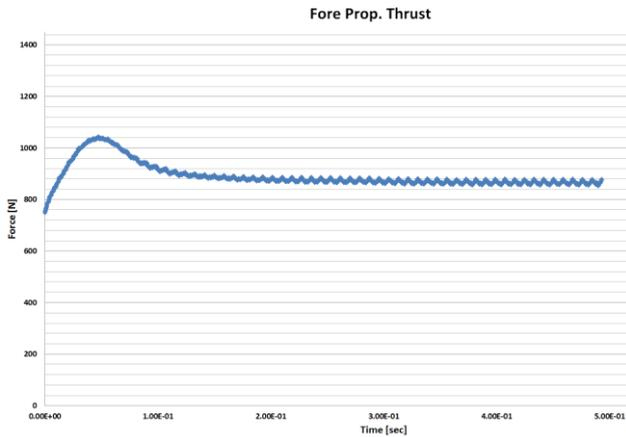
Figure 9. Fore Propeller Thrust fluctuations in time
