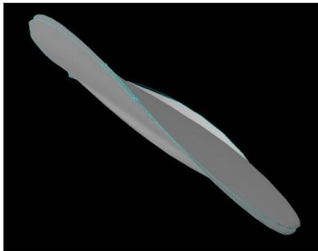
Figure 13. Forward blade pitch correction by 5 percent (view from blade top)
