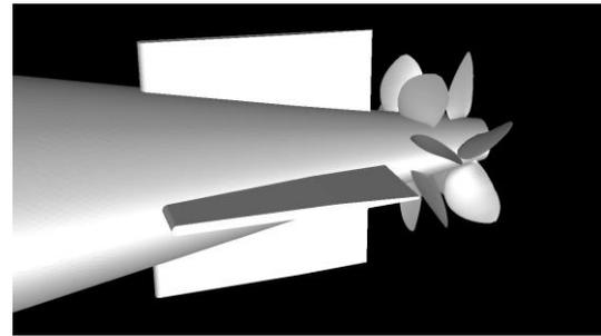
Figure 8. CRP Geometry from side-view
