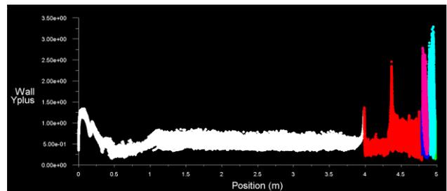
Figure 5. Boundary layer  $y^+$  value through axial position
