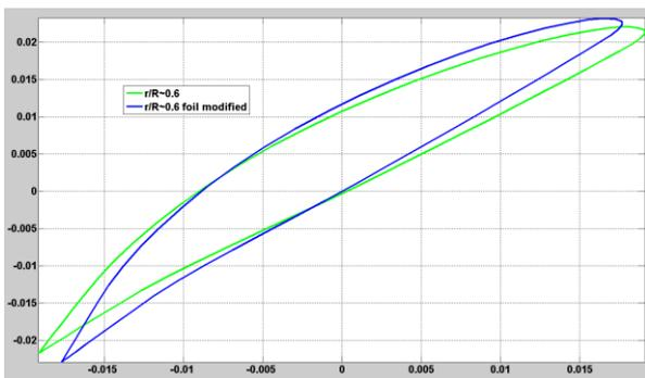
Figure 14. Forward blade pitch correction by 15 percent
