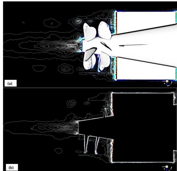
Figure 12. Vorticity (around 3000 1/s) distribution after using a) LES and b) URANS
