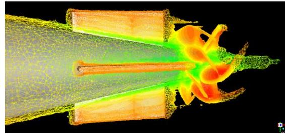
Figure 11. Vorticity distribution (around 200 1/s) shedding from appandages and blades into the flow domain
