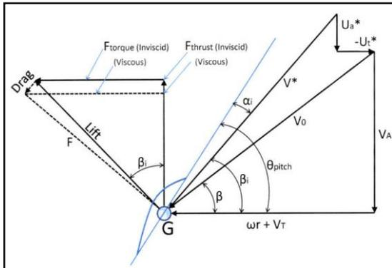
Figure 1. Velocity and angle definitions on blade profile (Epps 2010)
