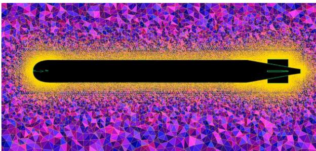
Figure 3. Fine mesh generated in flow volume
