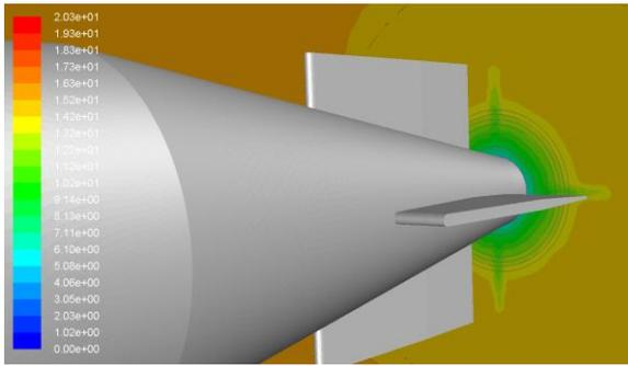
Figure 6. Nominal wake plotted on CRP inlet plane
