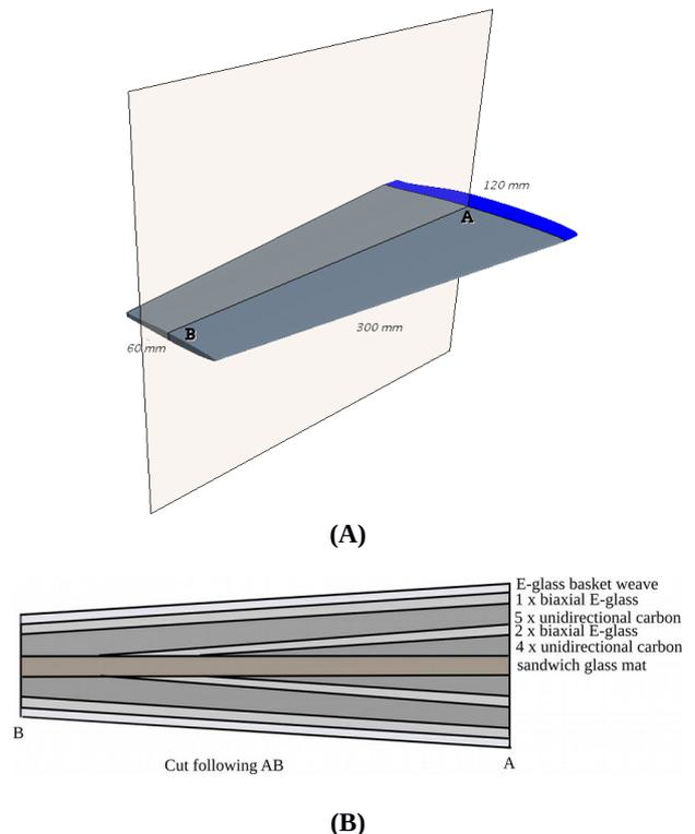
**Figure 2. (A) Geometry of the hydrofoil in dark gray, with its clamping disk in blue and (B) layers arrangement of the composite hydrofoil featuring the plies drops - cut following the mid-plane section from (A).**
