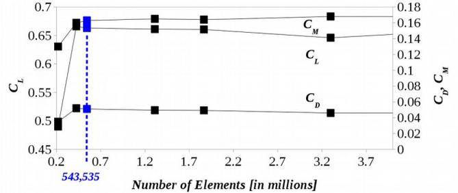
**Figure 8. Mesh convergence study using seven meshes for the configuration with  $8^\circ$  angle of attack and  $Re = 600,000$**
