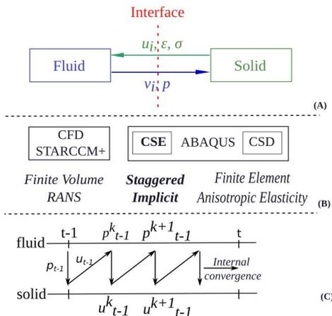
**Figure 7. (A) Principle of a fluid-structure coupling, (B) Numerical Codes and Methods used in this work, (C) Details of the Staggered Implicit Coupling Algorithm**
