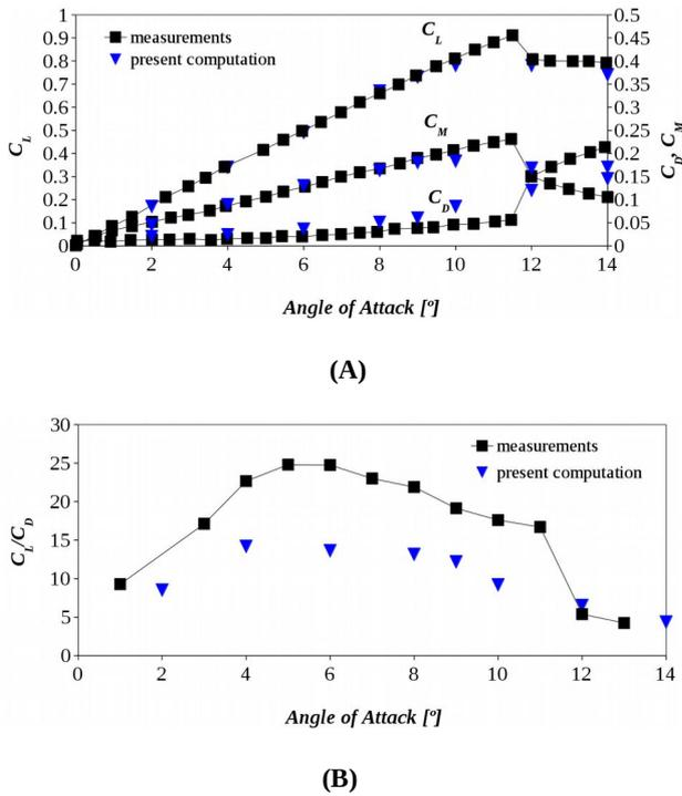
**Figure 9. (A) Comparisons between numerical computation and experimental measurements of Zarruk et al. 2014, on hydrodynamic coefficients for angles of incidence ranging from 0° to 14°, (B) performances curve.  $Re=600,000$**
