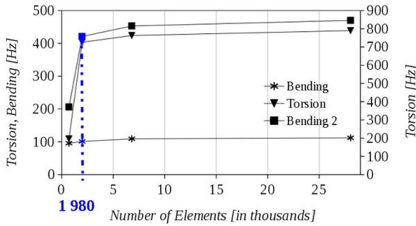
Figure 10. Structural Mesh Convergence Study on the First Three Modes
