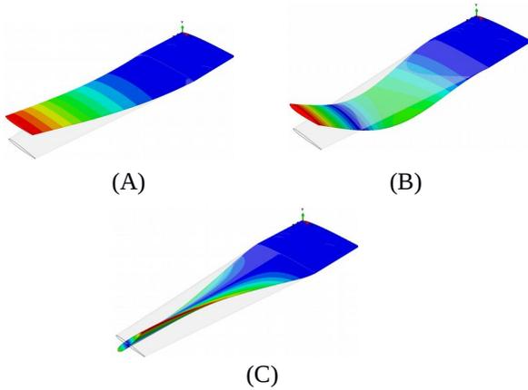
Figure 11. Frequency analysis of the aluminum hydrofoil (A) First bending mode, (B) Second bending mode and (C) First torsion mode
