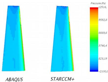
Figure 12. Validation of the transfer of pressure between the fluid solver and the structure solver,  $\alpha=8^\circ$
