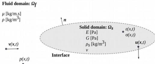
**Figure 3. Theoretical formulation of the fluid-structure interaction problem.**
