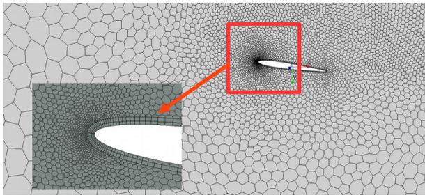
**Figure 5. Illustrations of the fluid domain mesh**
