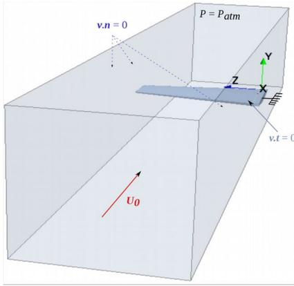
**Figure 4. Schematic illustration of the fluid domain and boundary conditions.**
