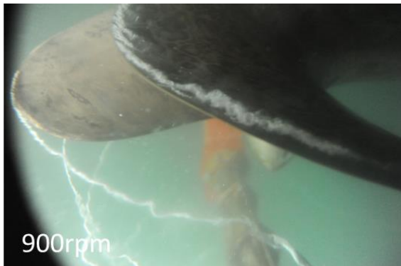
Figure 12 Full scale trial cavitation observation– 900 engine rpm.
