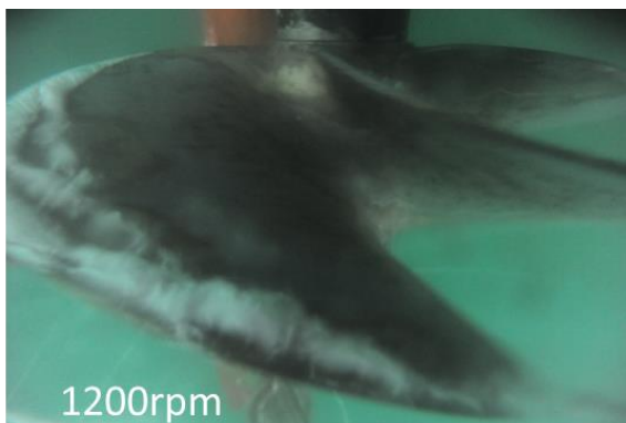
Figure 12 Full scale trial cavitation observation– 900 engine rpm.
