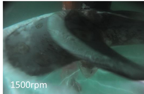
Figure 14 Full scale trial cavitation observation– 1500 engine rpm.
