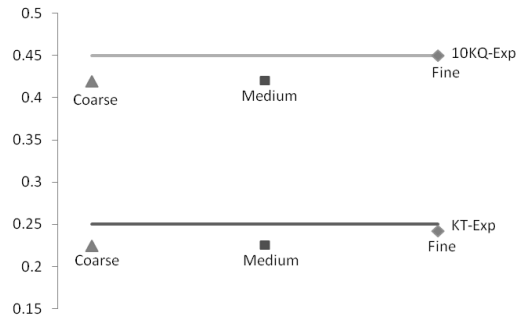
Figure 8 Comparison of convergence of CFD values and experiment results from coarse to fine mesh
