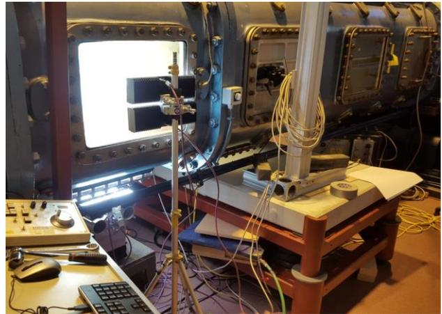
Figure 8: Picture of the cavitation tunnel test set-up.
