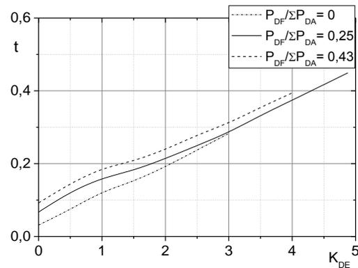
Figure 3. The relationships of thrust deduction factor  $t$  at various power ratios of bow ( $P_{DF}$ ) and stern ( $P_{DA}$ ) thruster units.
