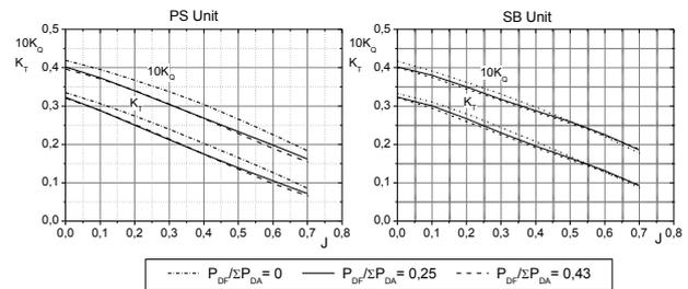
Figure 4. Thrust coefficient  $K_T$  and torque coefficient  $K_Q$  for SB and PS stern units versus advance  $J_V$  at various power ratios of bow and stern units.
