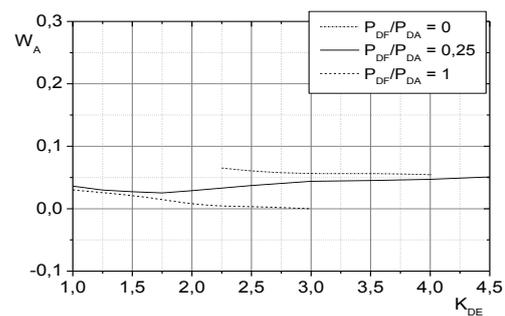
Figure 7. The relationships for wake coefficient of stern thruster units  $w_A$  at various ratios of power delivered to bow and stern units.
