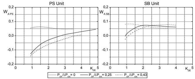
Figure 2. The relationships of wake coefficients  $w$  for SB and PS stern thruster units at various power ratios of bow ( $P_{DF}$ ) and stern ( $P_{DA}$ ) thruster units.
