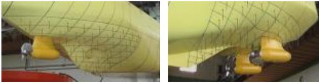
Figure 1. Thruster units installed on the model of Aker ARC 130A icebreaker.
