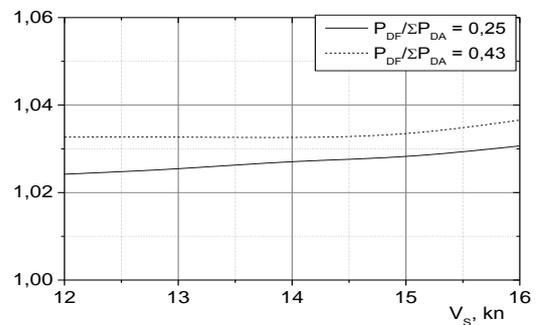
**Figure 11. The relationships of rotational frequencies of PS and SB stern units' propellers of Aker ARC 130A icebreaker during the operation of bow thruster unit.**
