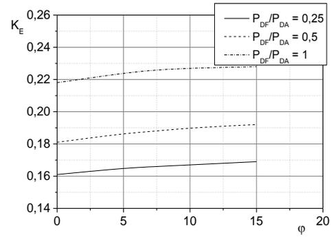
Figure 6. Total effective thrust coefficient  $K_E$  versus toe-out angle of bow units  $\varphi$  for various power distributions between bow and stern units in bollard pull mode.
