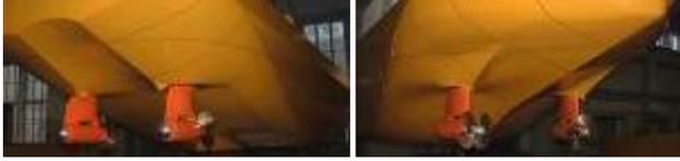
Figure 5. Thruster units installed on the model of icebreaker Aker ARC 124.
