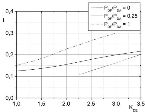
**Figure 8. The relationships for thrust deduction factor at various ratios of power delivered to bow and stern thruster units.**
