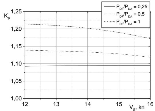
**Figure 10.  $K_P$  factor versus speed of Aker ARC 124 icebreaker with two bow thruster units.**
