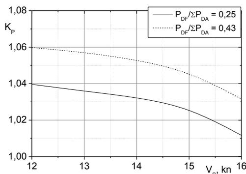
**Figure 9.  $K_P$  factor versus speed of Aker ARC 130A icebreaker with one bow thruster unit.**
