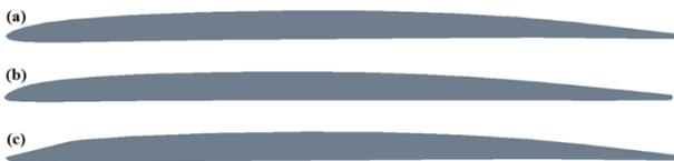
Figure 2 – Blade’s profile of the prototype propeller (a) and its two modifications
