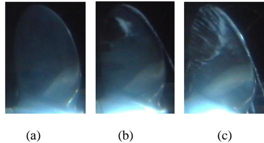
Fig.4. Cavitation on propeller blades at  $J=0.512$   $\sqrt{\sigma_n}=0.409$ . (a) – without roughness; (b) – with roughness  $\mu=3\mu\text{ m}$ ; (c) – with roughness  $\mu=30\mu\text{ m}$ .
