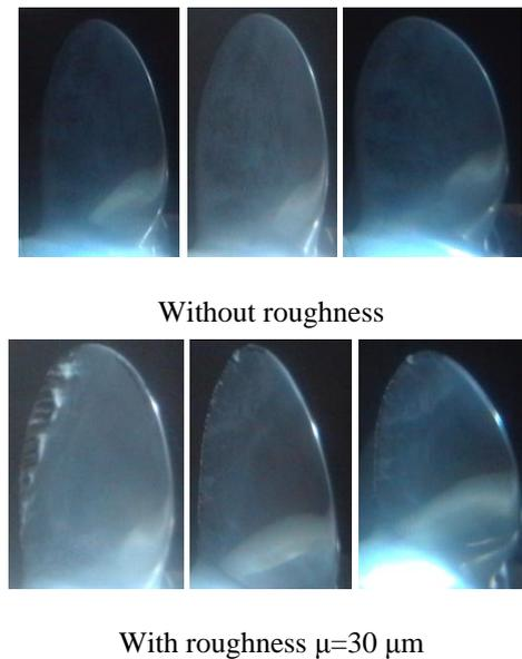
Fig.5. Propeller blade cavitation at  $\sqrt{\sigma_n}=0.470$  for different advance ratio  $J=0.539; 0.763; 0.906$ .
