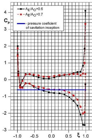
Fig.2 Pressure distribution over blade outline at various blade area ratios
