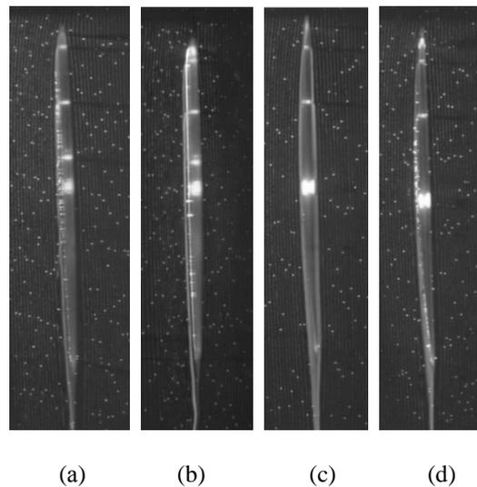
Fig.9. Test results of blade sections with and without roughness at  $2^\circ$  attack angle; (a), (b) – ice blade section without roughness and with roughness at leading edge, respectively; (c), (d) –NACA 66-mod section without roughness and with roughness at leading edge, respectively
