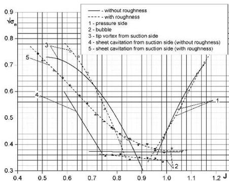
Fig.3. Distortion of the cavitation bucket due to artificial roughness applied on blades of passenger ship propeller
