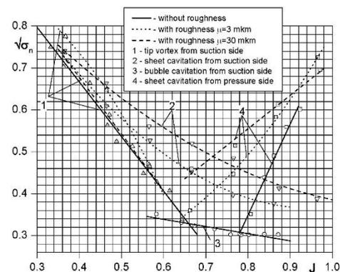
Fig.6. Effect of leading edge roughness on cavitation bucket of ice propeller.
