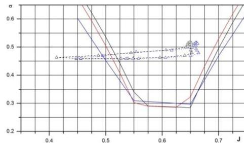
Fig. 12. Typical distribution of instantaneous advance ratios over one blade turn (different cavitation buckets correspond to cavitation at different propeller radii).
