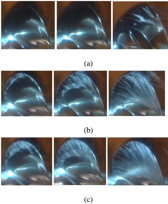
Fig.7. Non ice propeller blade cavitation at  $J=0.700$  and  $\sqrt{\sigma_n} = 0.600; 0.520; 0.420$ . (a) – without roughness; (b) – with roughness  $\mu=3 \mu\text{m}$ ; (c) – with roughness  $\mu=30 \mu\text{m}$ .
