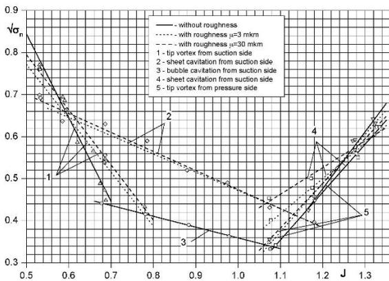
Fig.8. Effect of leading edge roughness on cavitation bucket of non-ice class propeller.
