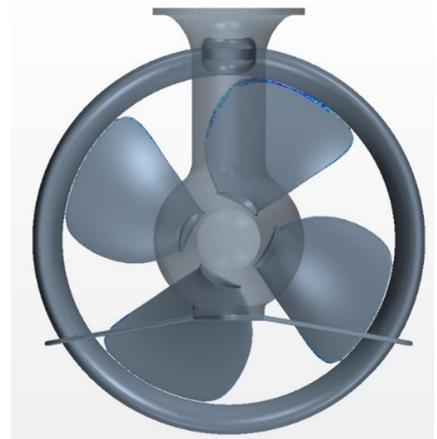
Figure 12: calculated cavitation pattern for model scale (top) and full scale
