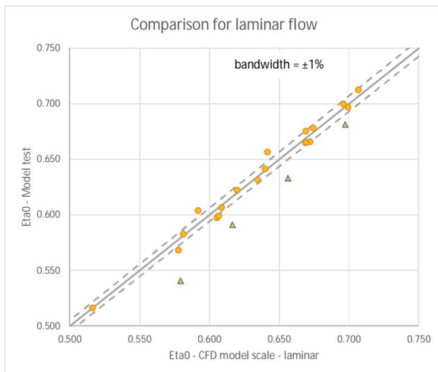
**Figure 5: comparison of open water efficiency at design point between CFD simulations based on laminar flow regime and model scale experiments for propellers with  $Re_{c-0.7}$  below  $6.0 \times 10^5$**
