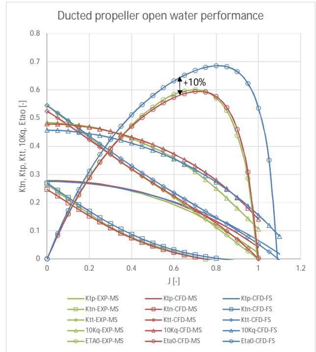
Figure 8: open water performance for ducted propeller based on model scale measurements, model scale CFD simulations and full scale CFD simulations
