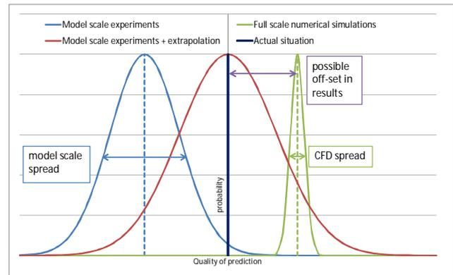
Figure 13: sketch of probability of accurate full scale performance predictions
