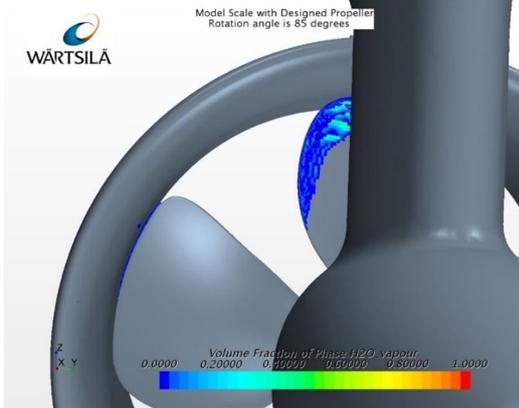
Figure 11: observed cavitation (top) and calculated cavitation on model scale
