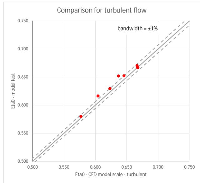
**Figure 6: comparison of open water efficiency at design point between CFD simulations based on turbulent flow regime and model scale experiments for propellers with  $Re_{c-0.7}$  above  $9.0 \times 10^5$**
