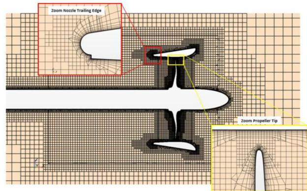
Figure 2: mesh example of ducted propeller
