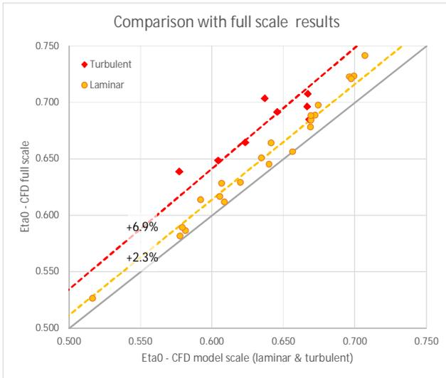
Figure 7: Reynolds scaling effect for propellers with laminar and turbulent flow regimes on model scale
