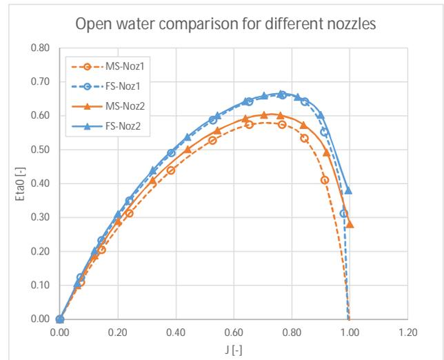
Figure 9: comparison of Reynolds scaling impact for 2 different nozzles
