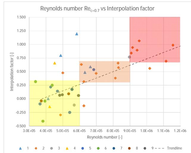
**Figure 4: evaluation of Interpolation Factor as function of local Reynolds number of 0.7R chord length**
