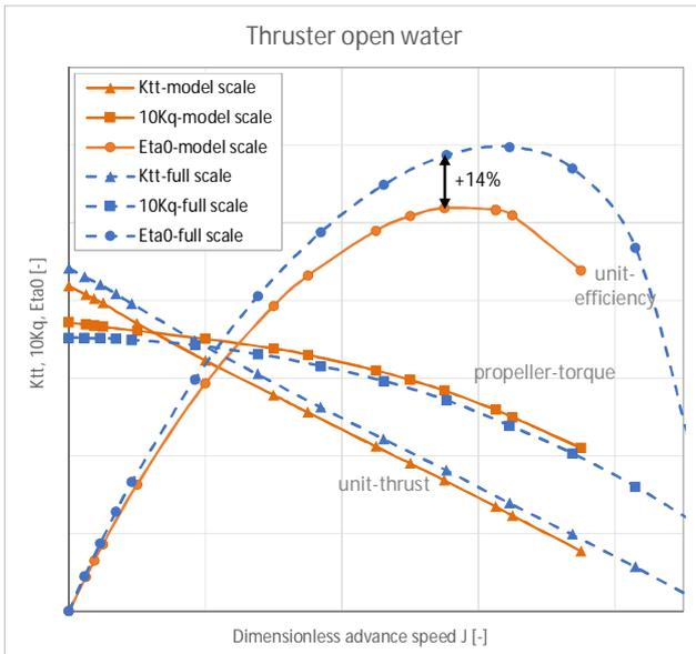
Figure 10: open water performance of azimuth thruster for model scale and full scale
