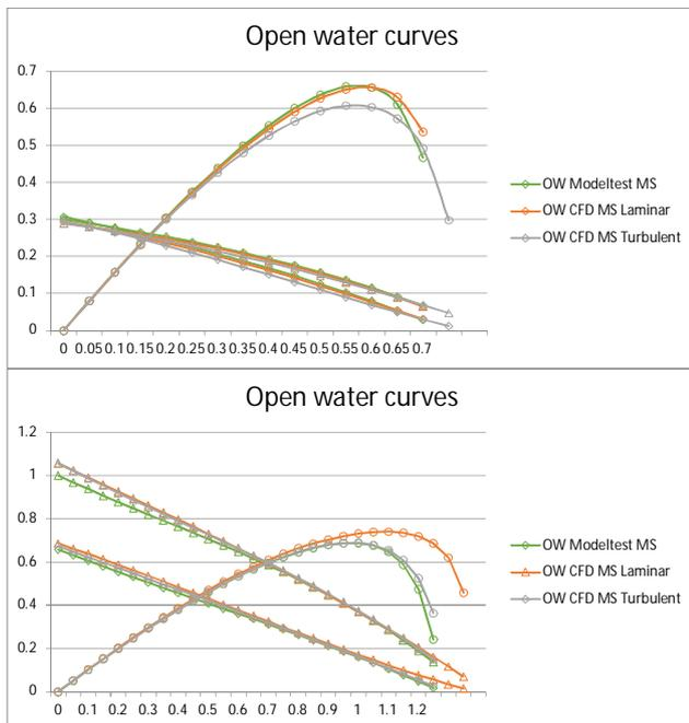
**Figure 3: open water comparisons of CFD results with model scale measurements based on laminar flow regime (top) and turbulent flow regime**
