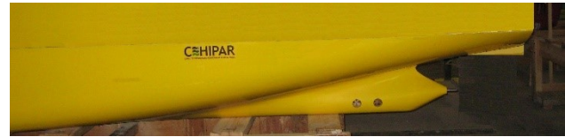
Figure 3. Stern of the ship model to carry out resistance test. Without appendages.
