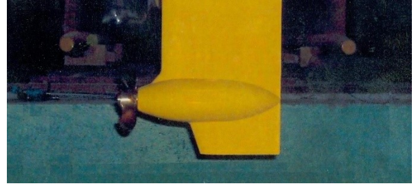
Figure 6. Open water test. Aft propeller in the POD housing.
