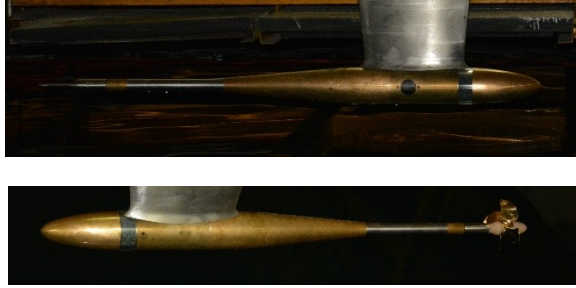
Figure 4. Fore propeller. Open water tests. Up, normal position; down, reversed flow.
