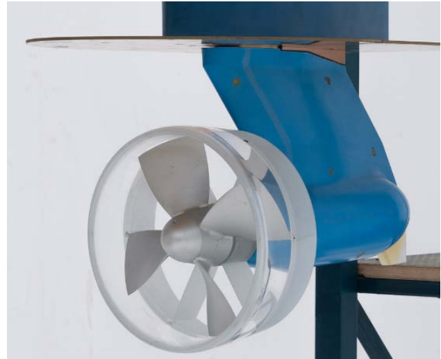
Figure 3: Photograph of the open water setup.
