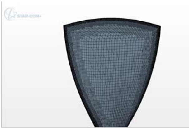
Figure 6: Mesh resolution on the propeller surface
