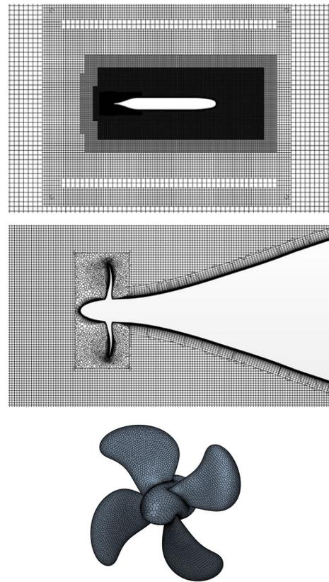
Figure 3. Grid distribution (a) near field region, (b) aft part boundary layer prism layer and propeller region mesh and (c) propeller surface mesh.
