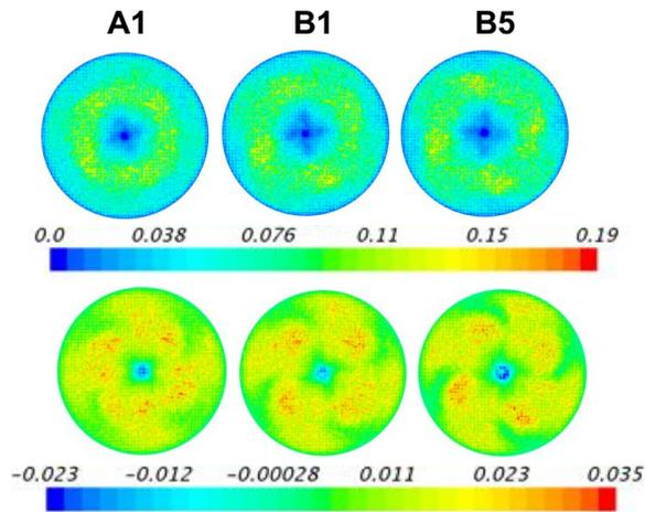
Figure 10. Distribution of the useful energy components for different propeller designs just behind the propeller (top) axial kinetic energy and (bottom) pressure work.
