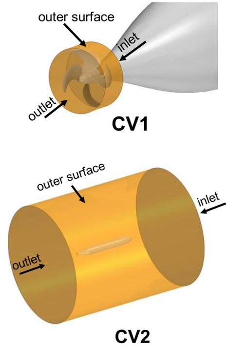
Figure 6. Two different control volumes (top) only containing the propeller, CV1, and (bottom) containing both the propeller and hull, CV2.
