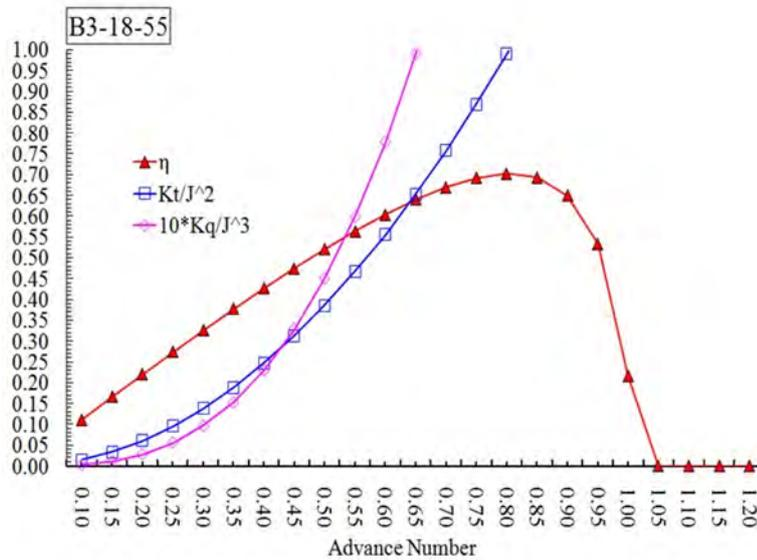
Figure 5: Propellers performance characteristic curves of new-model type 3B-18-55
