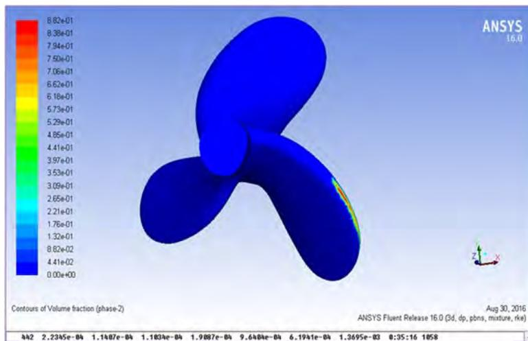
Figure 19: Contour plots of predicted volume fraction cavity patterns on suction (back) side at RPM 850,  $J_s = 0.701$  and  $\sigma_n = 1.386$  of New-model; Type 3B-18-55
