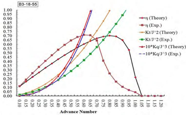
Figure 7: Comparison on the performance curves of inverse  $K_t$ ,  $K_q$  and  $\eta$ , New-model
