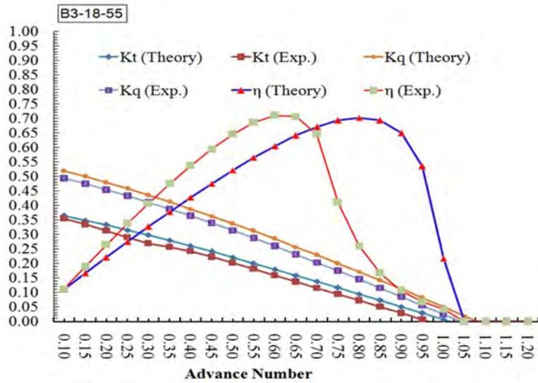
Figure 6: Comparison on the performance curves of  $K_t$ ,  $K_q$  and  $\eta$ , New-model
