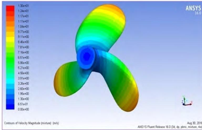
Figure 17: Contour plots of velocity at RPM 850,  $J_s = 0.701$  and  $\sigma_n = 1.386$  of New-model; Type 3B-18-55
