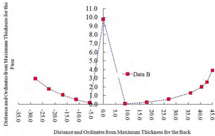
Figure 9: Chord distributions of the wide-chord tip blade
