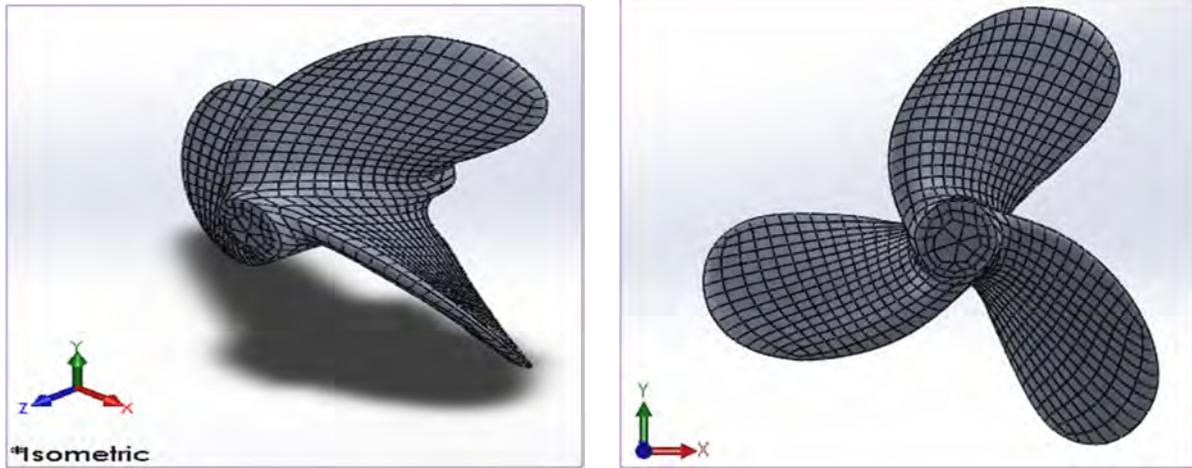
Figure 12: Illustration contours surface of blade New-model; Type 3B-18-55
