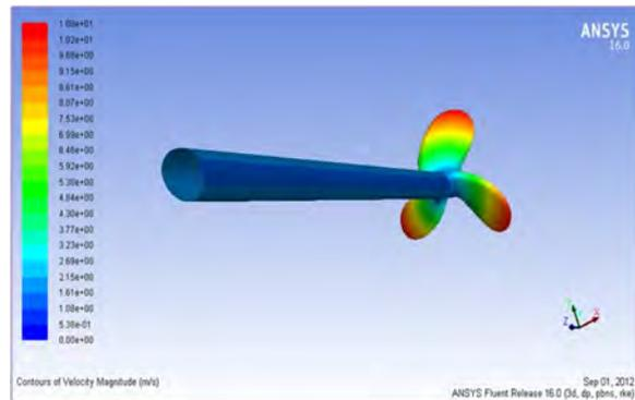
Figure 16: The computational domain of New-model propeller; Type 3B-18-55
