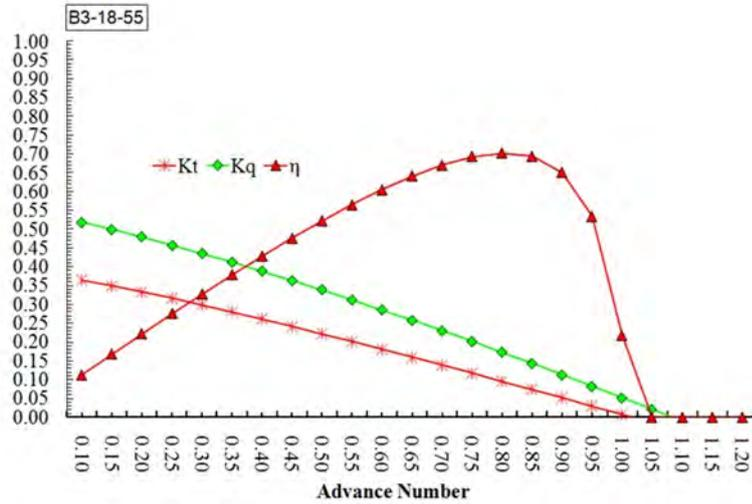
Figure 4: Propellers performance characteristic curves, new-model type 3B-18-55
