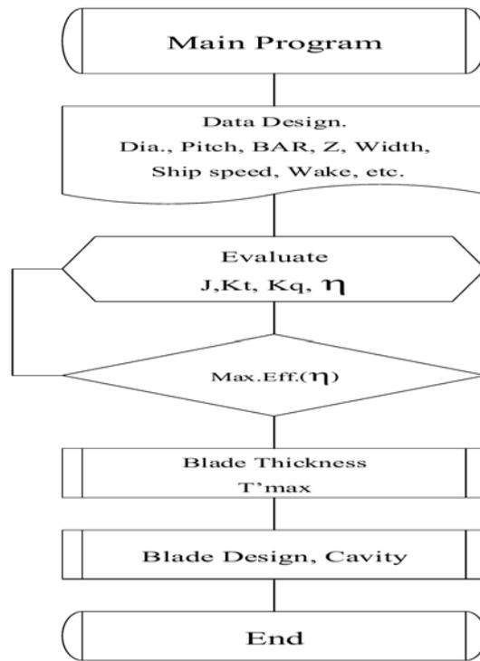
Figure 2: Flow-chart for the determination of an optimal propeller configuration.
