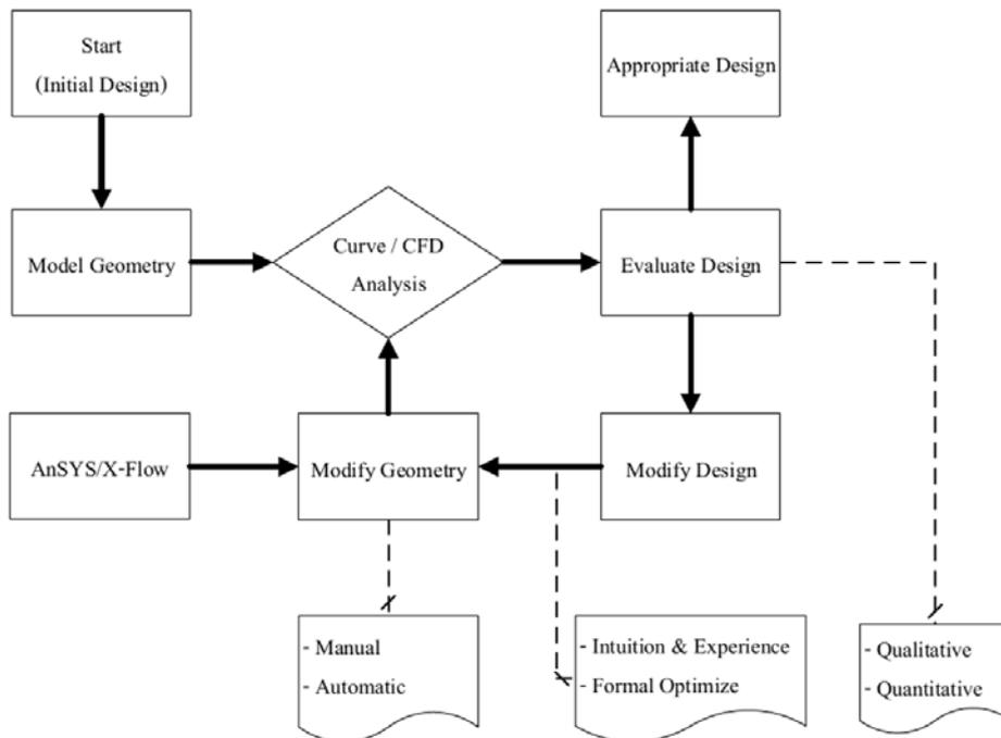
Figure 3: Conceptual design and analysis blade Model
