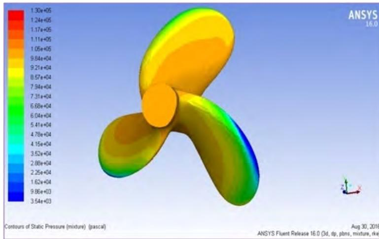
Figure 18: Contour plots of predicted static pressure patterns on suction (back) side at RPM 850,  $J_s = 0.701$  and  $\sigma_n = 1.386$  of New-model; Type 3B-18-55
