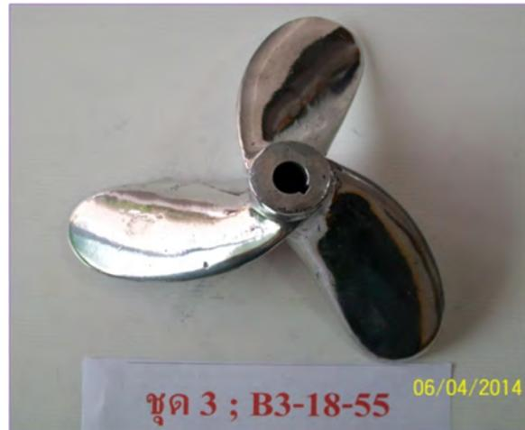
Figure 11: Casting blade of New-model; Type 3B-18-55
