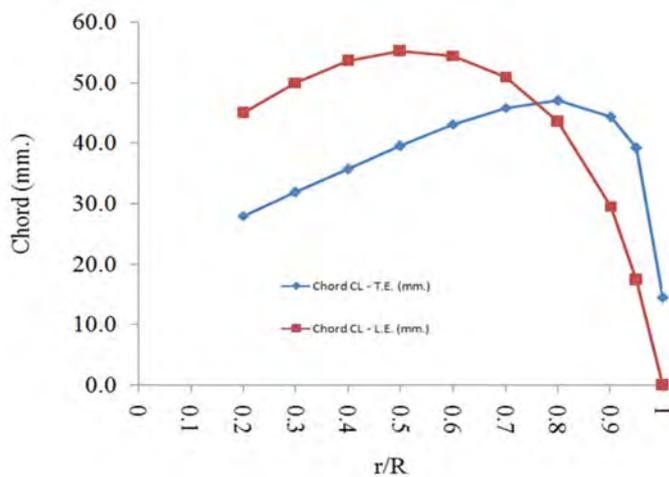
Figure 8: Chord distributions of the width-chord tip blade
