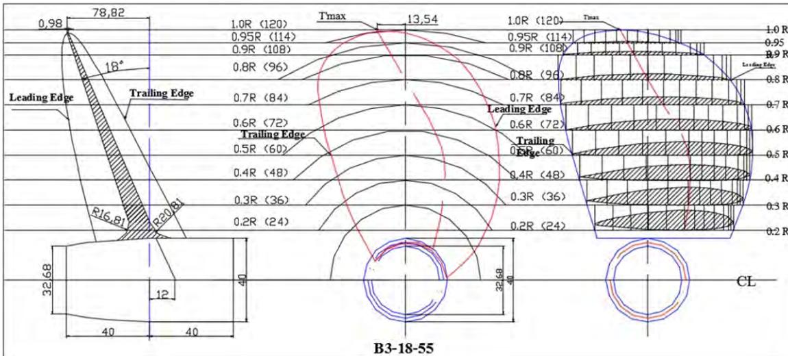
Figure 10: Drawing of propeller design, Type 3 Blades, Rake degree angle 18, Developed area 55
