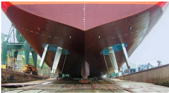
Fig. 3: Voith-Schneider propellers installed under the ship hull.
