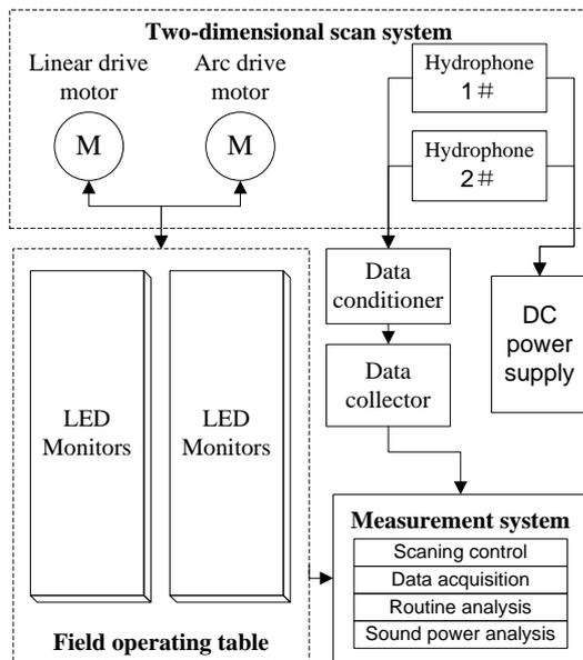
**Figure 6 Composition of the comparative test and analysis system for the noise of propulsion pumps**
