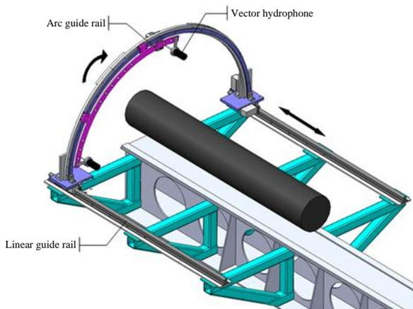
**Figure 7 Two-dimensional scanning motion mechanism**
