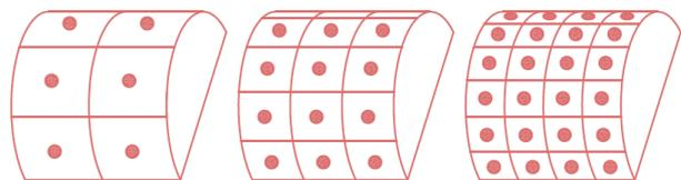
**Figure 3 Discrete sound intensity measurement**
