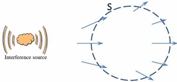
**Figure 1 Propagation of sound waves through the envelop surface from interference sources outside**
