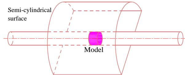
**Figure 2 The semi-cylindrical measuring surface**
