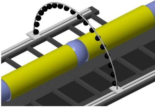
Figure 4 1-D scan using an array of hydrophones
