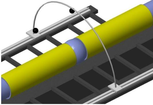
Figure 5 2-D scan using a single hydrophone
