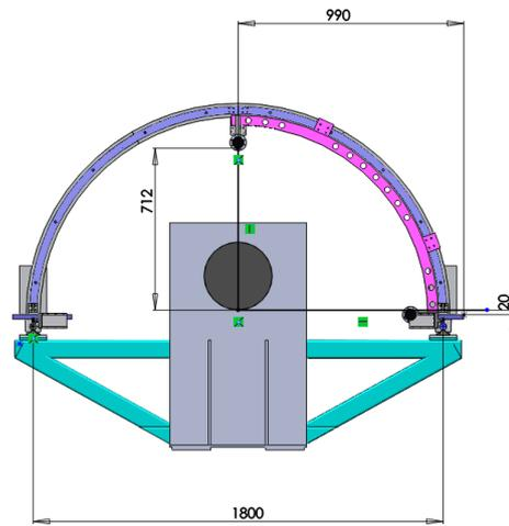
**Figure 8 Main dimensions of the scanning mechanism**
