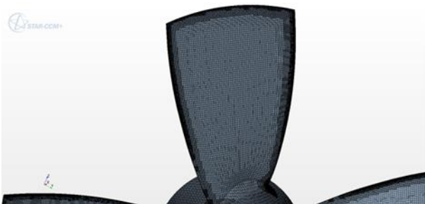
Figure 2: Mesh resolution on the propeller surface.
