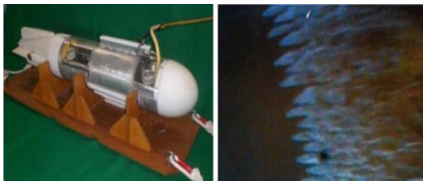
Figure 3: Towed underwater vehicle containing a camera (left photograph) and air bubble flow released from air injector of actual ship (right photograph).
