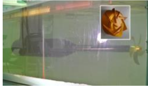
Figure 14: Facility to measure the propeller characteristics by reverse POT
