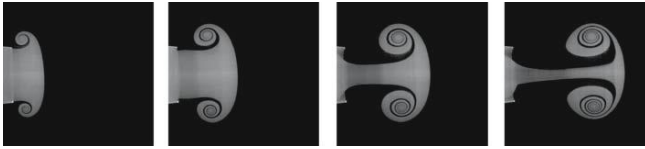
Figure 10: Vortex ring formation in the wake of a starting jet from the work by Olcay and Krueger (2008).
