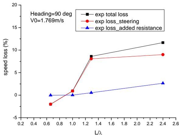
**Figure 5** Speed loss due to steering and added resistance in regular waves at a heading of 90 degrees.
