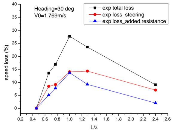
Figure 3 Speed loss due to steering and added resistance in regular waves at a heading of 30 degrees.
