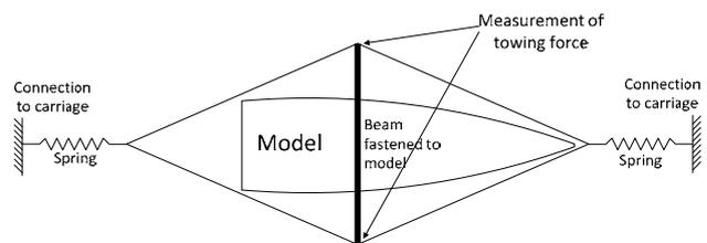
**Figure 1 Towing arrangement for seakeeping tests (set-up type 2)**
