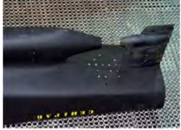
Fig. 5.3. Dummy model for cavitation tests with CRP-POD system.
