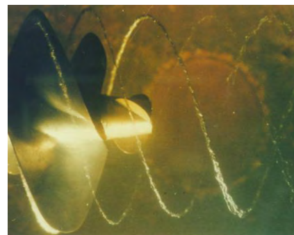
(b) Scheme B propeller with PBCF
