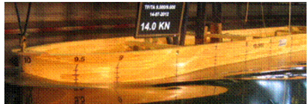
Figure 9. Wave profile at design speed ( V_s = 14.0 knots)
