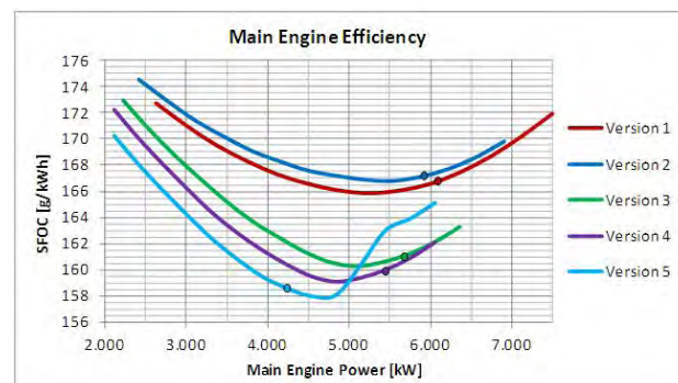
Figure 12. Main Engines SFOC and NCR (Source: MAN B&W)
