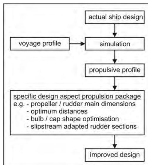
Figure 1: Schematic design approach
