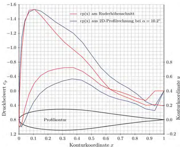
Figure 7: Equivalent pressure distribution
