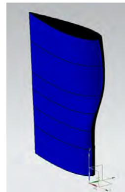
Figure 9: S-shaped rudder blade
