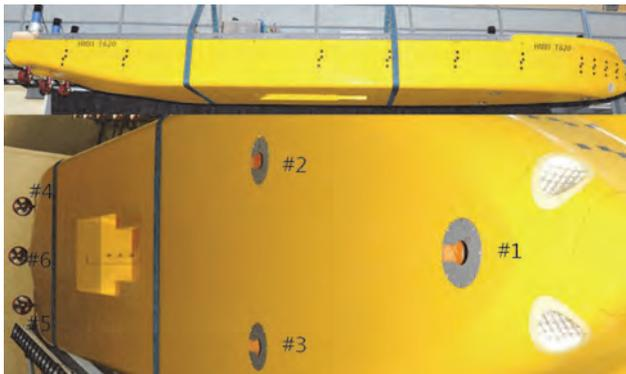
Figure 8 Arrangement of 6 azimuth thrusters
