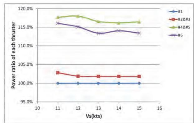
Figure 10 Power ratio of each thruster group (in constant revolution mode)
