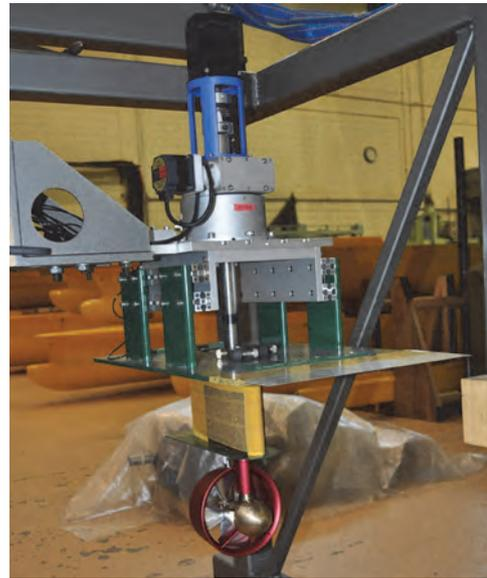
**Figure 3 Overall view of model azimuth thruster**
