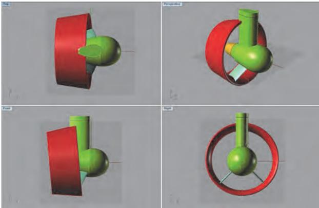
**Figure 1 Duct/housing/strut of azimuth thruster**
