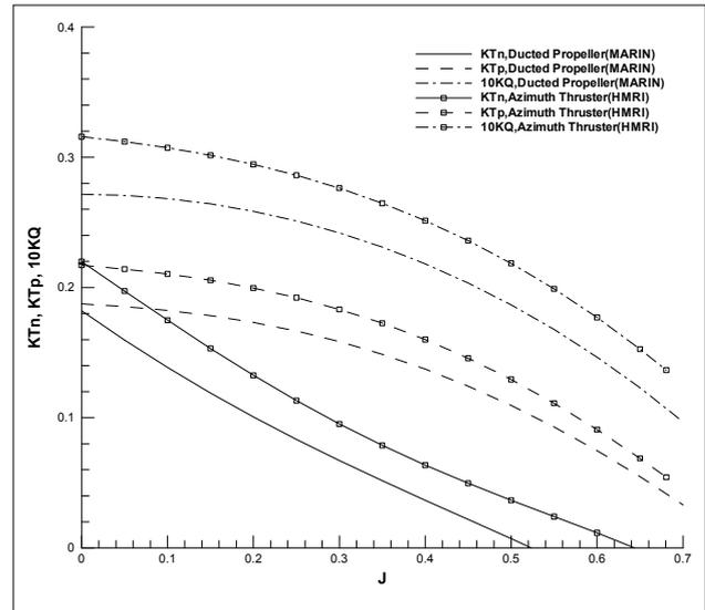
Figure 6 Open water characteristics of azimuth thruster
