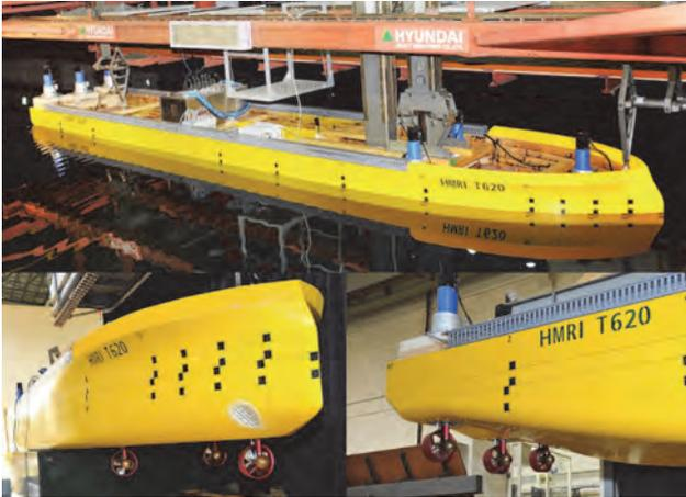
Figure 4 Overall and forward/after bottom view for propulsion test setup
