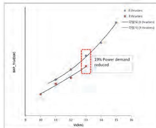
**Figure 13 Comparison of power in 6 & 3 thruster mode**
