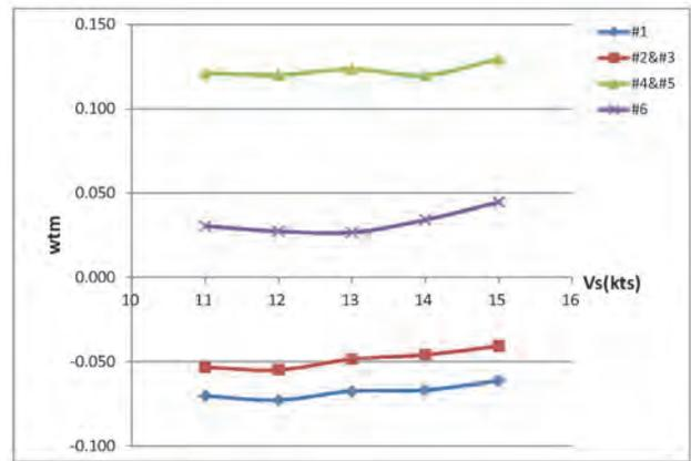
Figure 9 Wake fraction of each thruster's group
