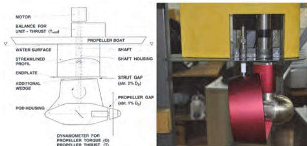
**Figure 2 Test setup for open water test of azimuth thruster**
