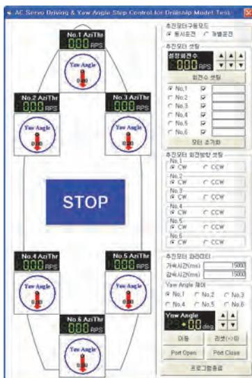
Figure 5 Integrated system for controlling propeller revolution and yaw angle of azimuth thruster
