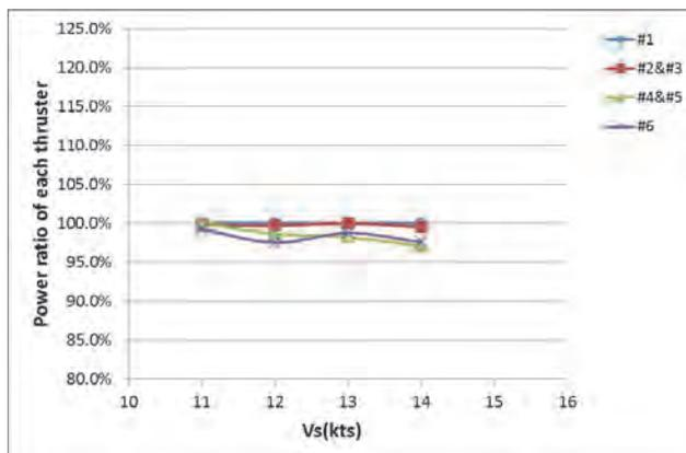
**Figure 11 Power ratio of each thruster group (in constant power mode)**
