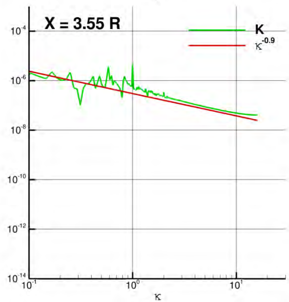
Figure 13: J = 0.45 - Numerical PSD of the kinetic energy at different stations downstream the propeller.
