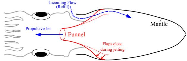
Figure 3: Diagram of squid anatomy showing separate inlet and outlet locations.
