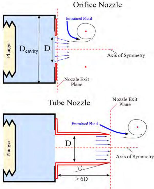
Figure 2: Schematic diagram of the thruster layout and different possible nozzle arrangements.
