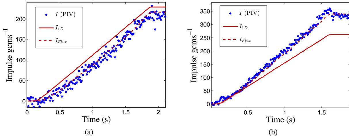
Figure 8: Total jet impulse is shown as a function of pulsation time for both parallel (a) and converging (b) starting jets. For both jet flows the piston velocity is  $u_p = 7\text{cm/s}$  and the jet stroke ratio is  $L/D = 7$ .  $I_{1D}$  represent the values calculated from the 1D slug model (3),  $I_{Flux}$  are the values calculated from the exact velocity profiles (2), and  $I(\text{PIV})$  are the values measured directly from PIV data (4).
