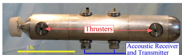
Figure 1: A prototype vehicle using the squid inspired thrusters of this investigation. The novel thruster provides the vehicle with accurate maneuvering capabilities without compromising the streamlined shape (Krieg et al. (2011)).
