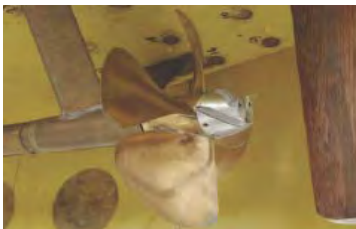
Figure 28. PBCF in cruise liner
