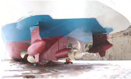
Figure 38. Hybrid Cruise Liner: pushing type Fixipod and two pulling type Pods
