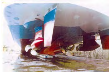
Figure 17. Well streamlined headbox
