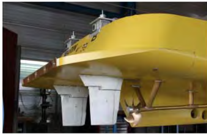
Figure 9. Example of a long ducktail with an interceptor plate fitted to a large cruise liner.
