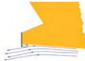
Figure 8. Operation principle of an interceptor plate
