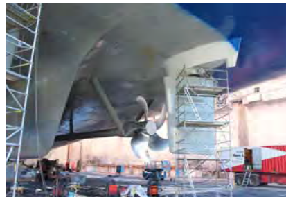
Figure 19. Big headbox above flap type rudder with ice knife.
