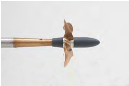
Figure 27. Typical OW-tests for propeller. The testing direction to the right.
