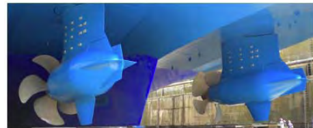
Figure 29. Two modern X-tail pods
