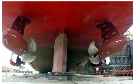
Figure 31. 4 pods in big cruise liner
