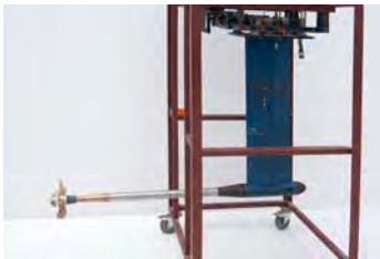
Figure 26. Reverse OW-tests for PBCF. The testing direction to the right.
